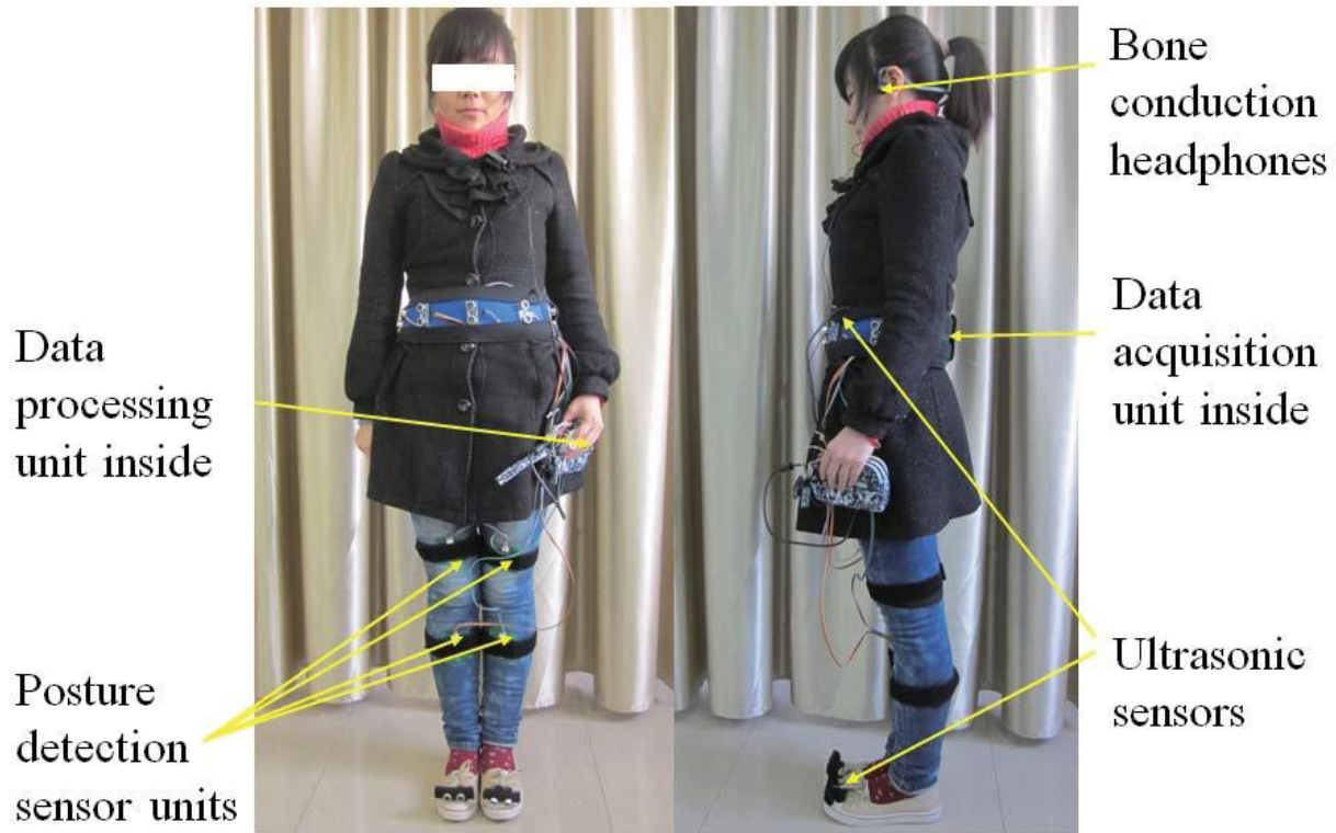
Fig. 2.3 An Electronic Travel Aid Based on Multi-Sensor Fusion Using Extended Kalman Filter
