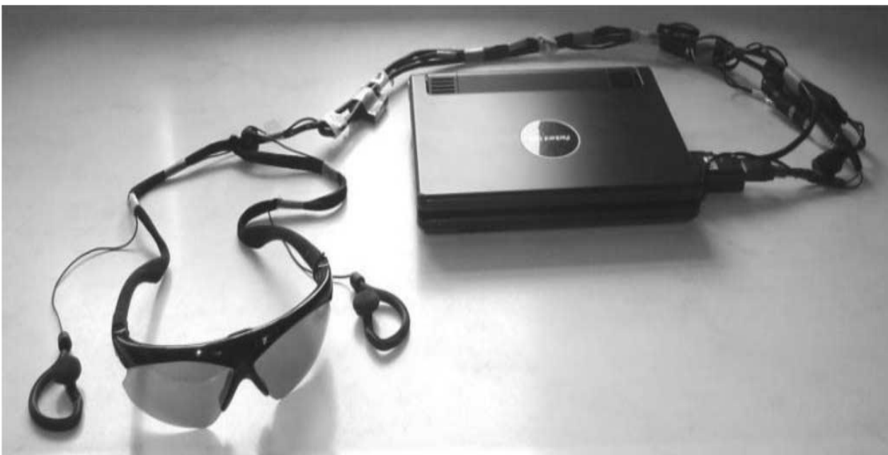
Fig. 2.7 voice— “Seeing with sound” system
