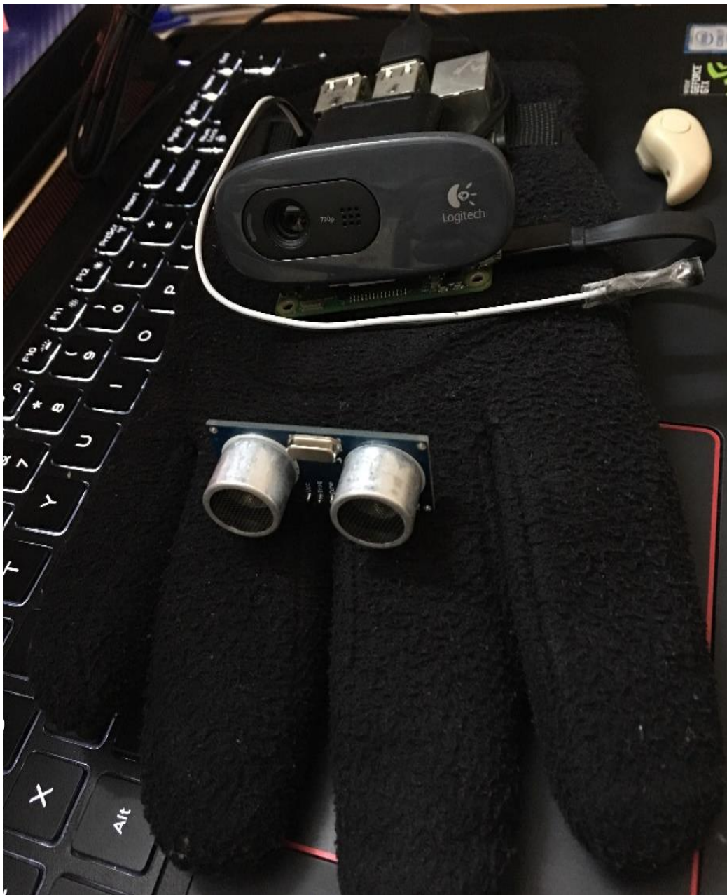
Fig.5.9 Assembled Computer vision and Obstacle avoidance device with Bluetooth Headset
