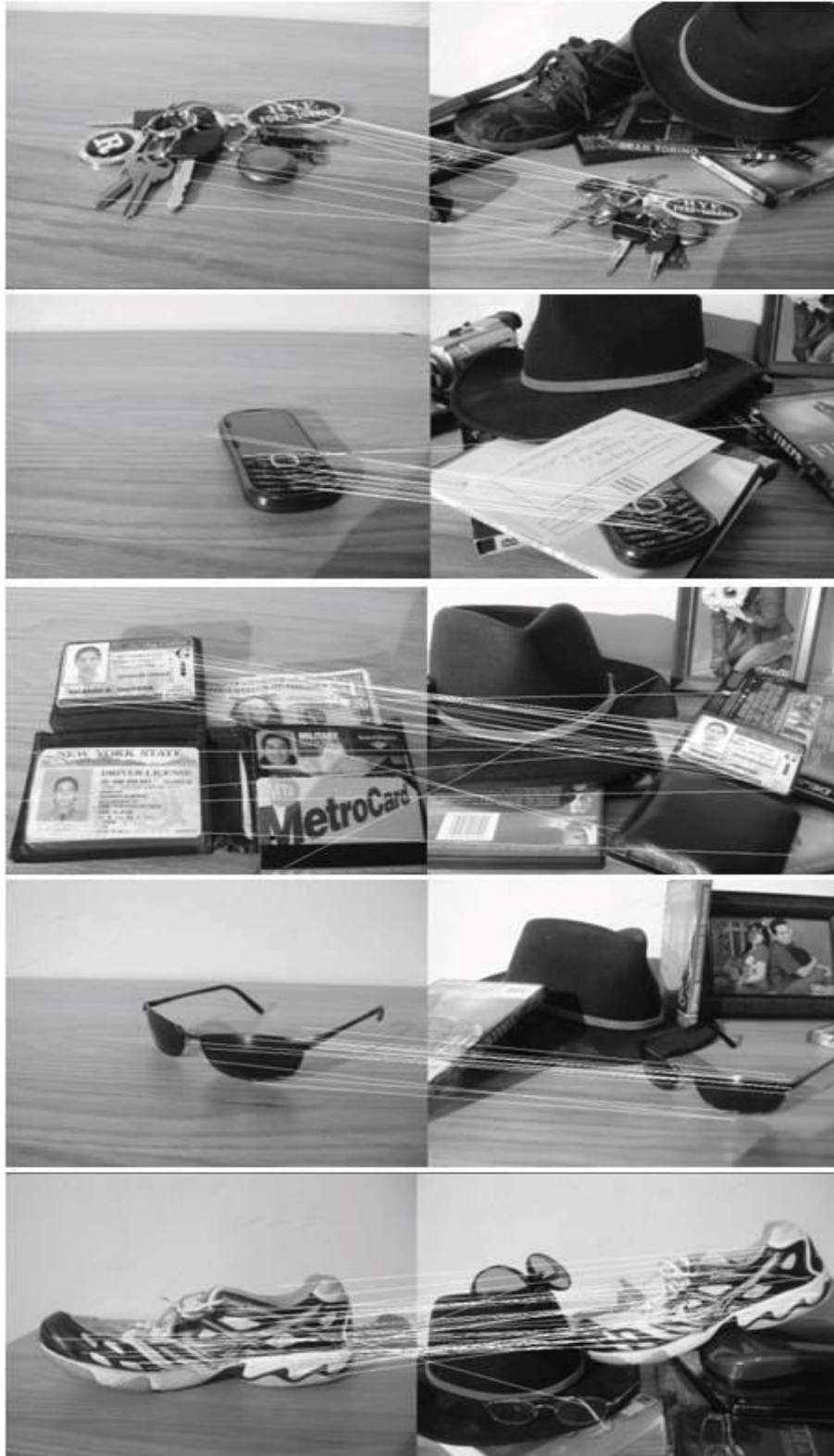
Fig. 2.9. Matching between reference and test images in the presence of cluttered background under various conditions, keys, cell phone, sunglasses, sneaker, and wallet.
