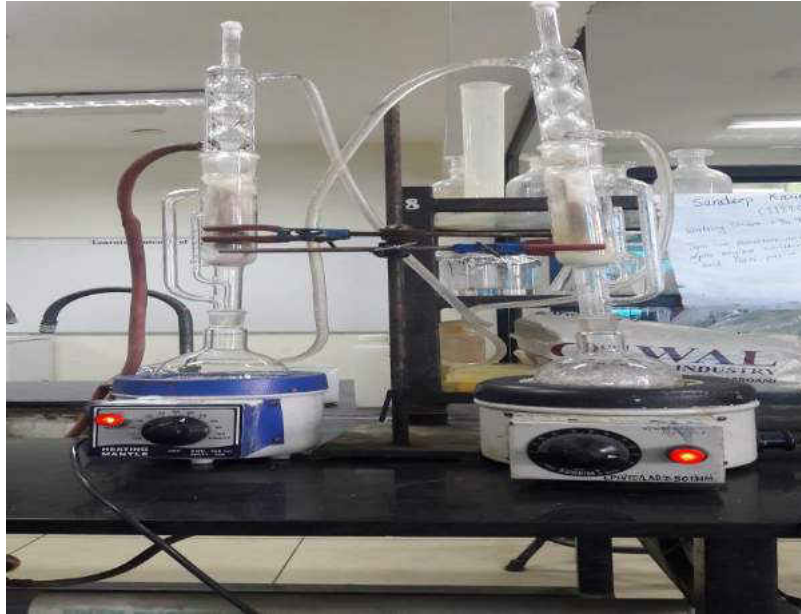
Figure 8: Soxhlet apparatus for preparation of plant extract
