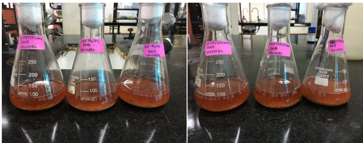
Figure 8: Immobilized yeast cells were added to the sample after 6 days of treatment by Trichoderma reesei .
