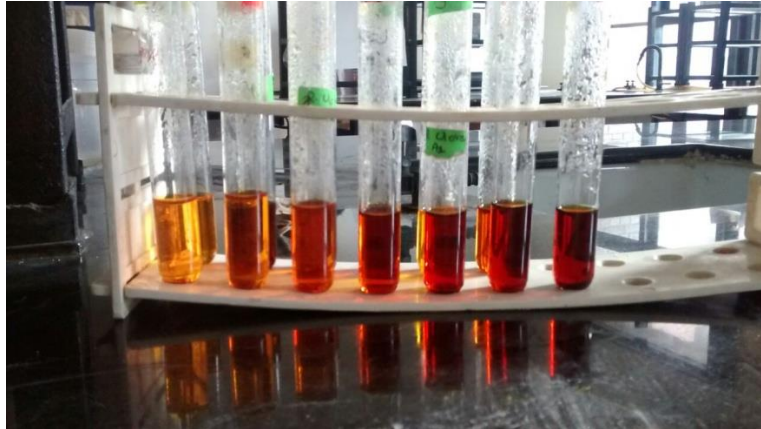
Figure 9: DNS test to know the glucose concentration in the sample
