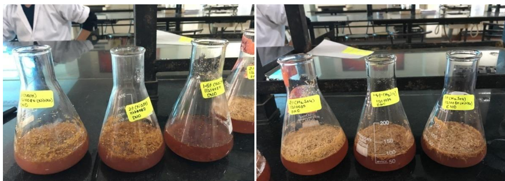
Figure 6: The sample added to the Mandels medium and then incubated for hydrolysis.
