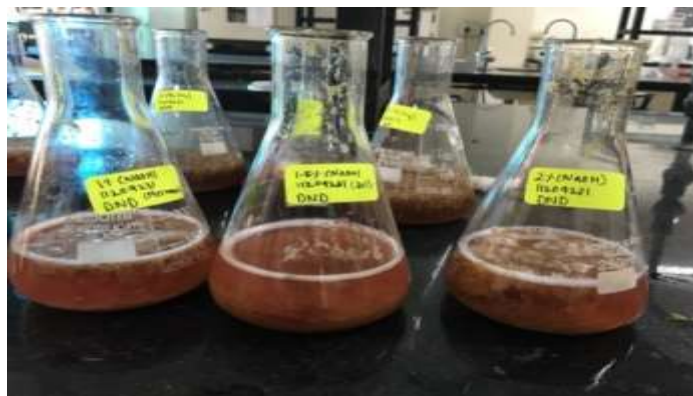
Figure 4. Fermentation media added to the pretreated wheat straw with NaOH and inoculated with enzyme.
