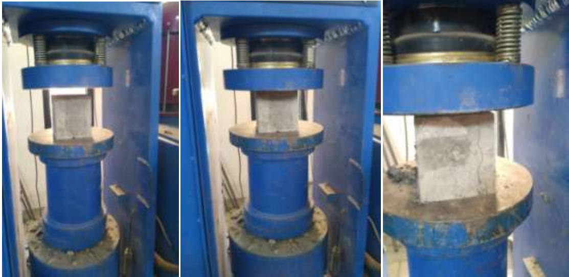
Figure 4.0 sample during compressive testing
