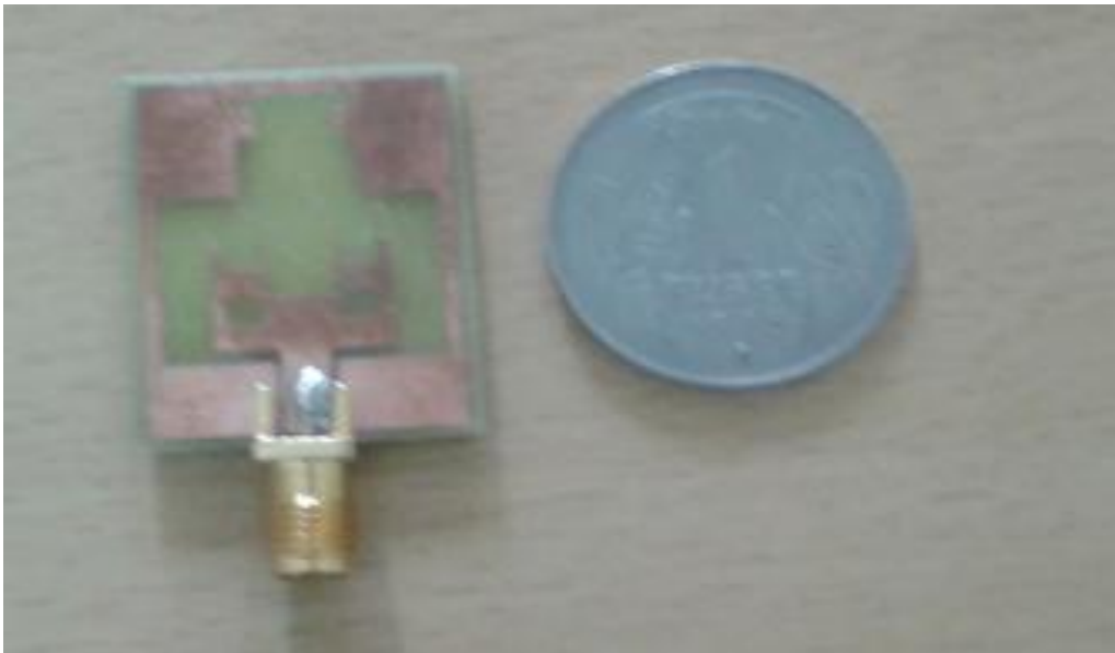
Fig 10.16 Fabricated antenna design
