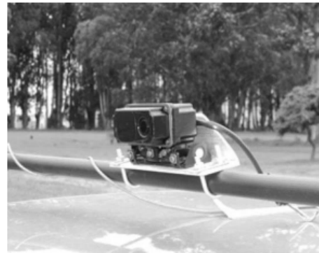
Fig. 2.17 - LIDAR mounted on top of the vehicle.
