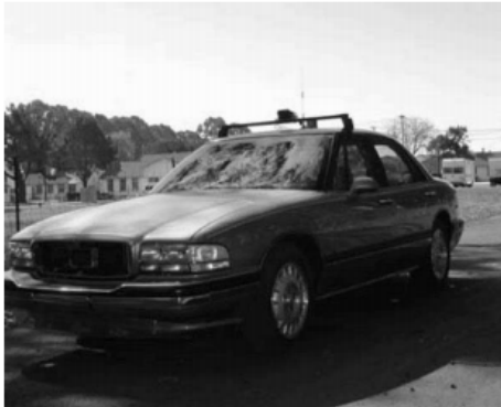
Fig. 2.17 - LIDAR mounted on top of the vehicle.
