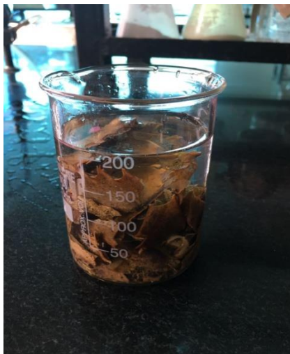
Figure 6.3.4 : represents crab shells were broken into small pieces and placed in a beaker filled with water
