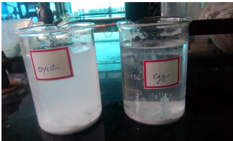
Figure 6.2.2 : represents HA formed at the bottom of the beakers from oyster and egg shells respectively
