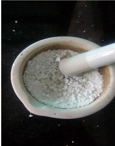
Figure 7.1.1 : (a) and (b) represents oyster shells after calcination were crushed by using mortar and pestle and amorphous powder was produced using grinder
