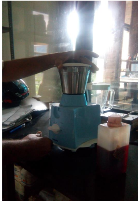
Figure 7.1.1 : (a) and (b) represents oyster shells after calcination were crushed by using mortar and pestle and amorphous powder was produced using grinder
