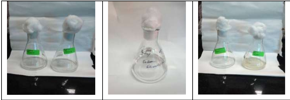
Figure no.7. Plastic films from the YPD agar plates were taken out with help of forceps and dipped in 50ml of 70% ethanol in different flasks and incubated in shaking incubator for 2 hours.
