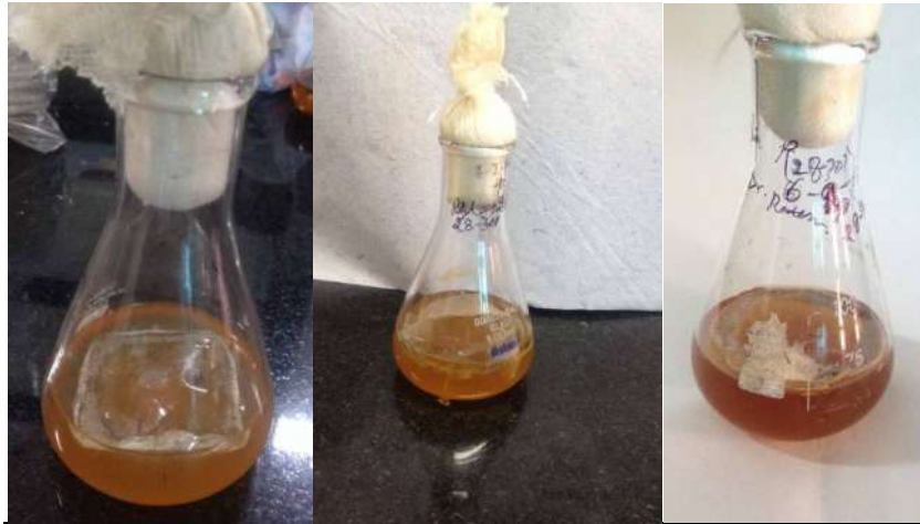
Plastic film degradation by RR fungi after 12, 22 and 36 days.
