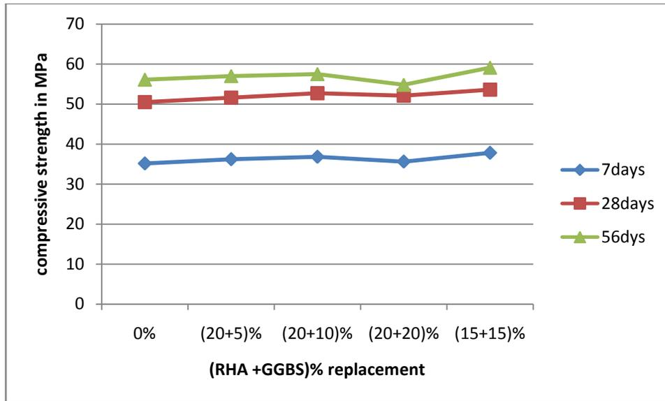
**Figure 7.2: Compressive strength of SCC mixes at various ages**
