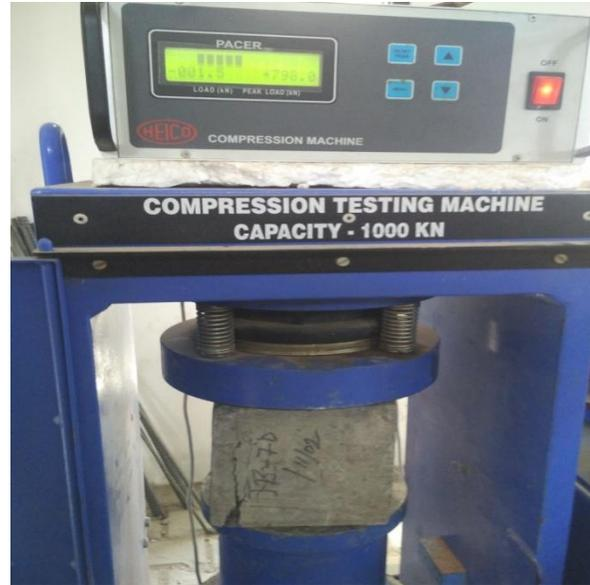
**Plate 6.7: Setup for Compressive strength showing concrete failure**
