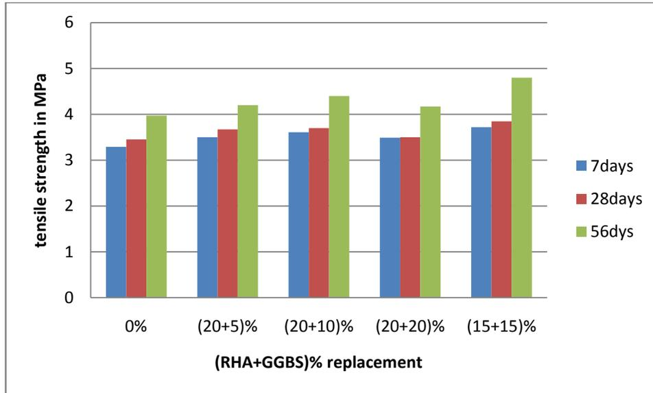
**Figure 7.3: Split tensile strength of SCC mixes at various ages**
