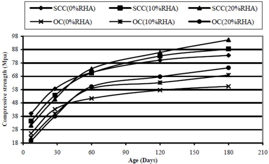
Figure 3.1 Compressive strength with w/b ratio 0.40 (Ahmadi *et al.*, 2007)
