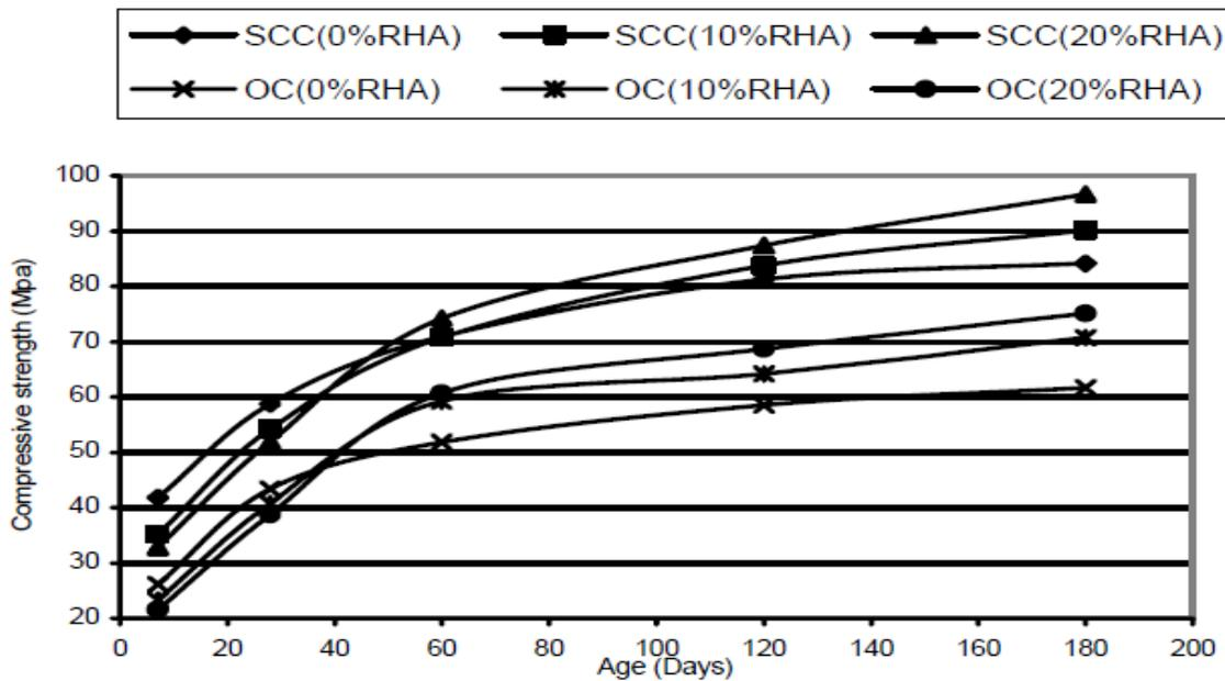
Figure 3.2 Compressive strength with- W/b ratio 0.35 (Ahmadi *et al.*, 2007)
