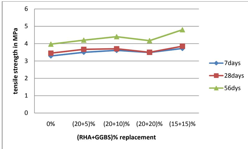
**Figure 7.4: Split tensile strength of SCC mixes at various ages**
