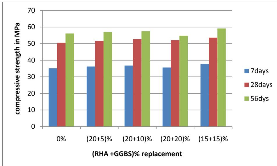
**Figure 7.1: Compressive strength of SCC mixes at various ages**
