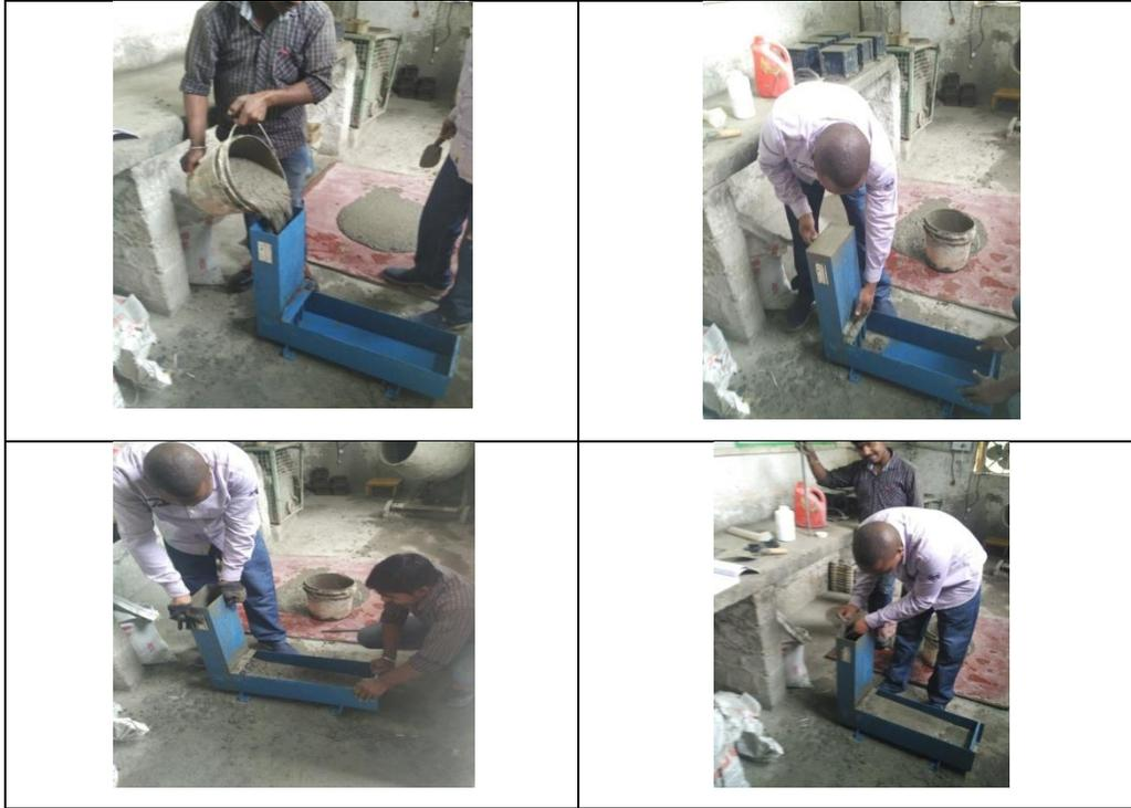
**Plate 6.4: L-box test process**
