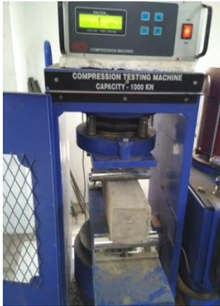
Plate 6.9: Setup for flexural before failure
