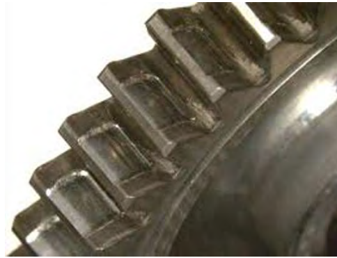
Figure 2.10: Plastic Flow in Gear
