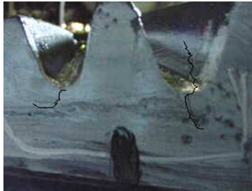
Figure 2.8: Fatigue breakage in gear tooth
