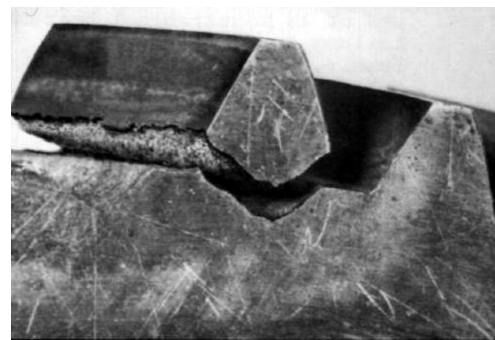
(b) Complete Tooth Breakage [10]
