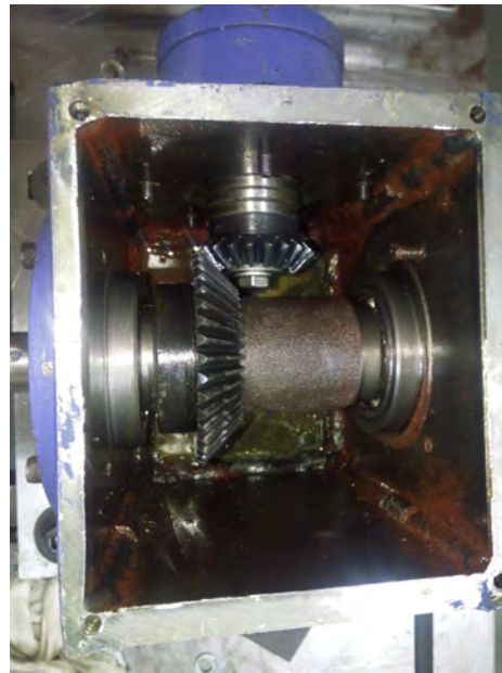
Figure 3.6: Top view of the straight bevel gearbox
