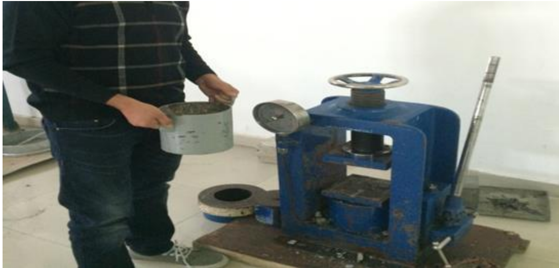
Figure 4.6.2 : Aggregate crushing test machine
