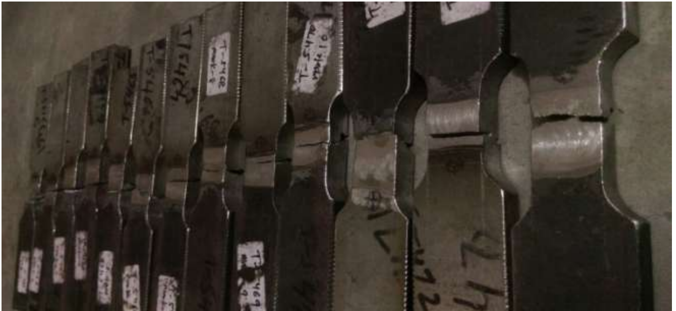
Figure 3.4 The location of fracture of the samples.
