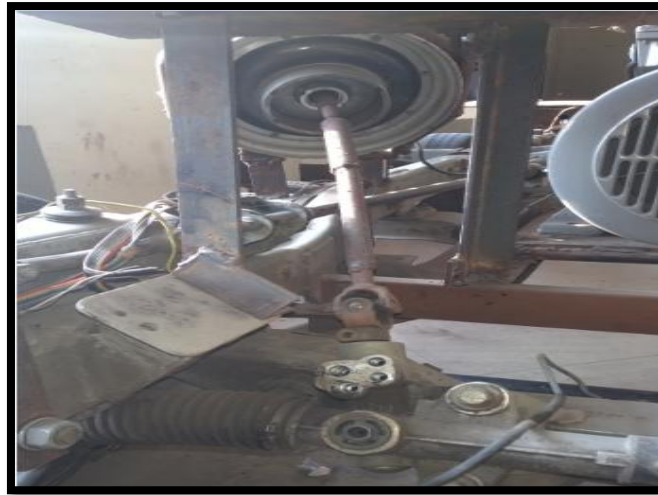
Figure:4.6 DC hub motor attached with the vehicle chassis
