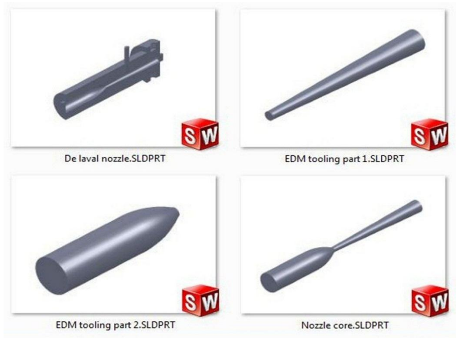
FIGURE 21 CAD MODELS SHOWING THE NOZZLE AND THE EDM TOOLING DESIGN
