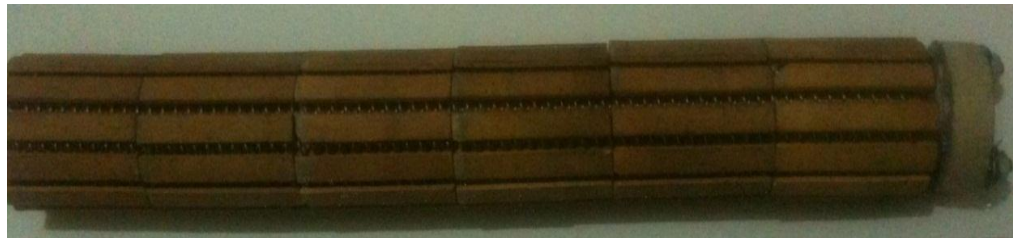
FIGURE 24 PHOTOGRAPH OF MANUFACTURED GAS HEATER
