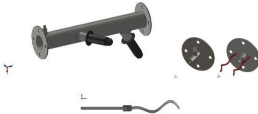
FIGURE 17 CAD MODELS OF GUN CASING AND MOUNTINGS
