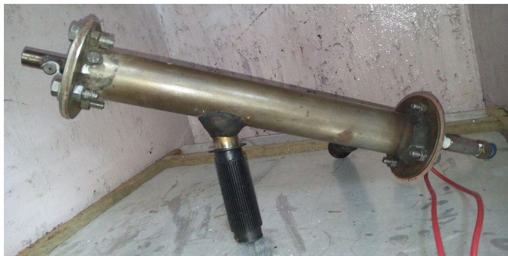
FIGURE 25 PHOTOGRAPH OF GUN CASING AND MOUNTINGS
