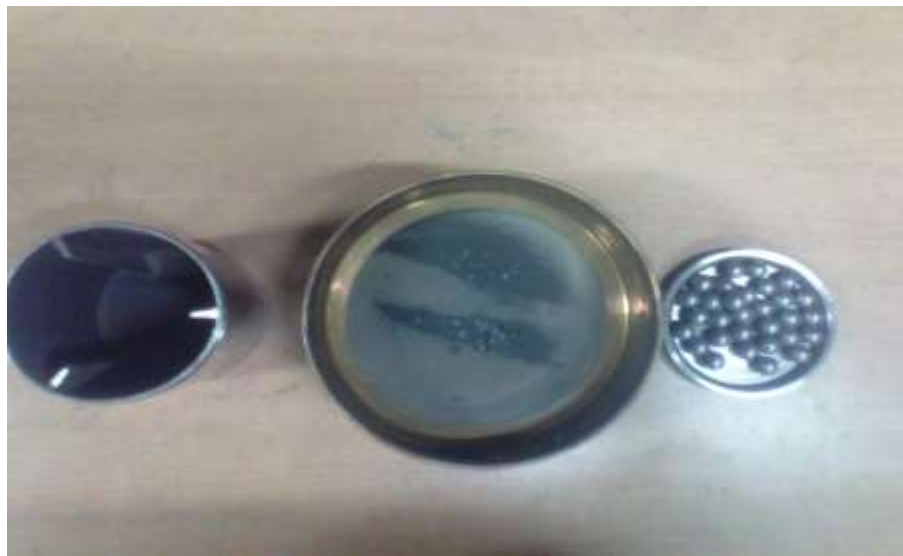
Fig 14 Ball mill with tungsten carbide ball for mixing of powders homogeneously
