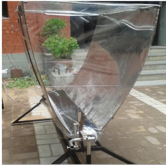
Figure 9 Fabricated 2-D Compound Parabolic Concentrator
