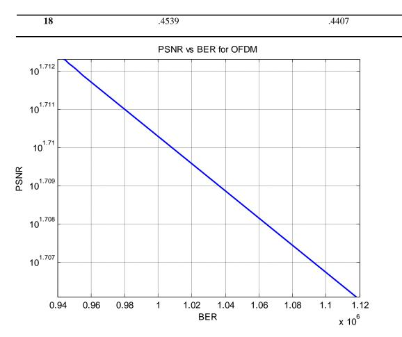
Figure 6-3-5 PSNR vs BER plot for transmitted and reconstructed image with OFDM
