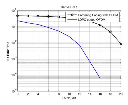
Figure 4-3-8 Performance Analysis of Hamming COFDM and LDPC coded OFDM with 256 FFT
