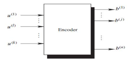
Figure 4-2-2 Convolutional Encoder
