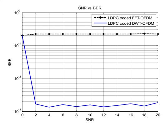
Figure 6-3-19 SNR vs BER plot for fused and compressed image transmitted with LDPC coded FFT-OFDM system and LDPC coded DWT-OFDM system
