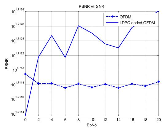
Figure 6-3-12 SNR vs PSNR plot for fused and compressed image transmitted with OFDM system and LDPC coded OFDM system
