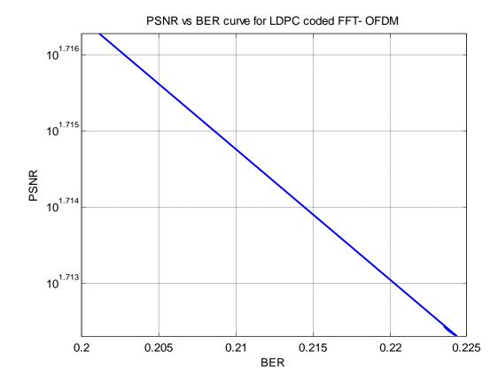
Figure 6-3-17 PSNR vs BER plot for transmitted and reconstructed image with LDPC coded FFT-OFDM
