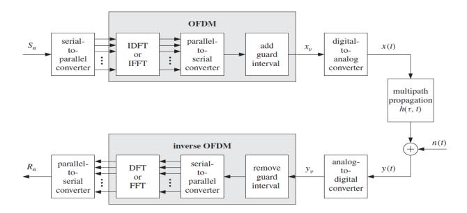
Figure 3-4-1 Digital multi-carrier transmission system applying OFDM
