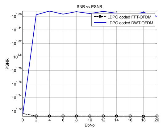
Figure 6-3-20 SNR vs PSNR plot for fused and compressed image transmitted with LDPC coded FFT-OFDM system and LDPC coded DWT-OFDM system
