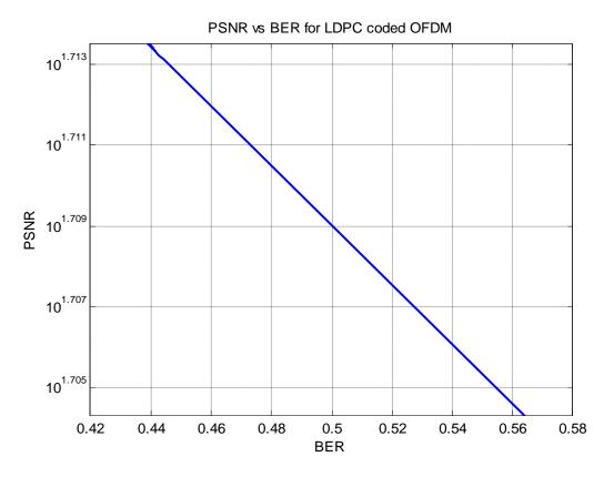
Figure 6-3-6 PSNR vs BER plot for transmitted and reconstructed image with LDPC coded OFDM
