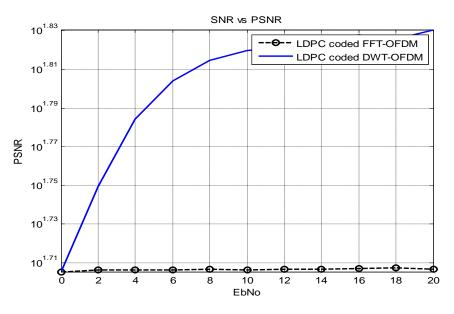
SNR vs PSNR plot for fused and compressed image transmitted with LDPC coded FFT-OFDM system and LDPC coded DWT-OFDM system
