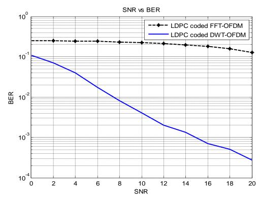
Figure 6-3-15 SNR vs BER plot for fused and compressed image transmitted with LDPC coded FFT-OFDM system and LDPC coded DWT-OFDM system
