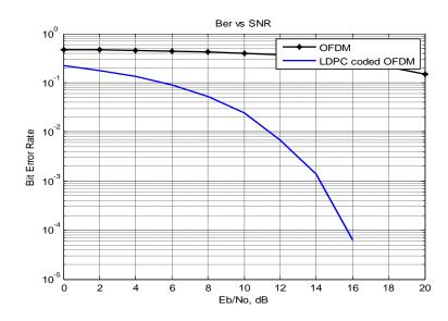
Figure 4-3-3 Performance Analysis of OFDM and LDPC coded OFDM with 64 FFT
