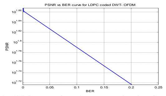
Figure 6-3-18 PSNR vs BER plot for transmitted and reconstructed image with LDPC coded DWT-OFDM
