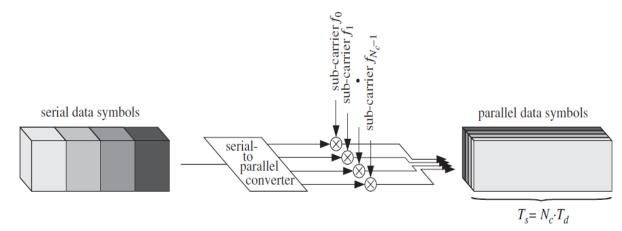
Figure 3-2-1 Multi-carrier modulation system with  $N_C = 4$  sub-channels
