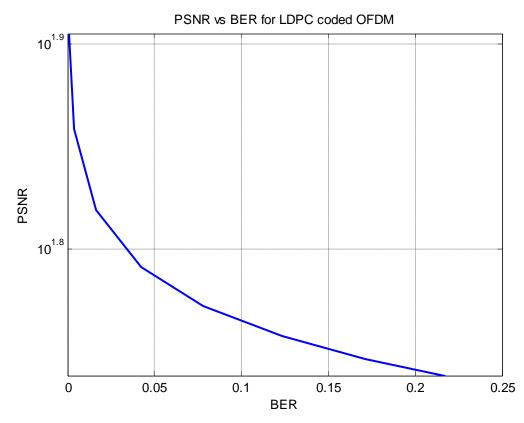
Figure 6-3-2 PSNR vs BER plot for transmitted and reconstructed image with LDPC coded OFDM
