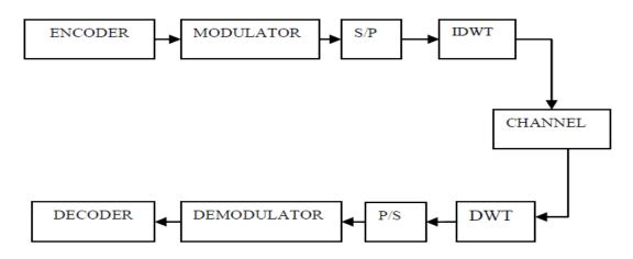
Figure 3-6-1Block diagram for DWT-OFDM
