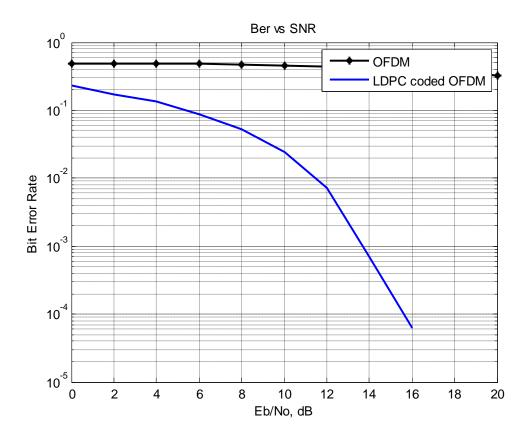
Figure 4-3-7 Performance Analysis of OFDM and LDPC coded OFDM with 256 FFT
