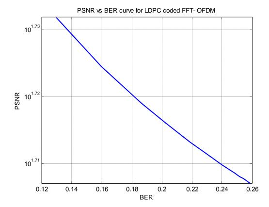
Figure 6-3-13 PSNR vs BER plot for transmitted and reconstructed image with LDPC coded FFT-OFDM
