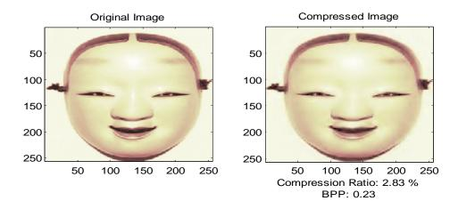
Figure 5-3-3 Example of SPIHT Compression
