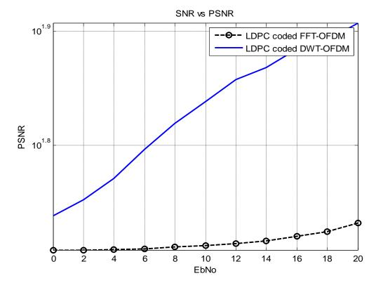
Figure 6-3-16 SNR vs PSNR plot for fused and compressed image transmitted with LDPC coded
