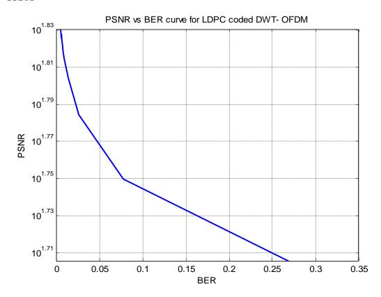
Figure 6-3-22 PSNR vs BER plot for transmitted and reconstructed image with LDPC coded DWT-OFDM
