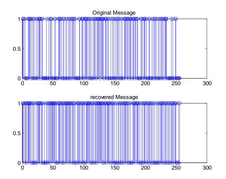
Figure 3.5.2 Original and Recovered Data from OFDM
