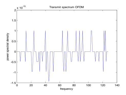
Figure 3.5.1 Transmit Spectrum of OFDM
