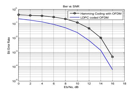
Figure 4-3-4 Performance Analysis of Hamming COFDM and LDPC coded OFDM with 64 FFT
