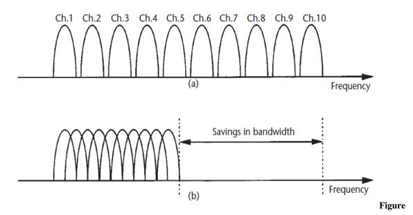
3-2-2 Concept of the OFDM signal: (a) FDM and (b) OFDM
