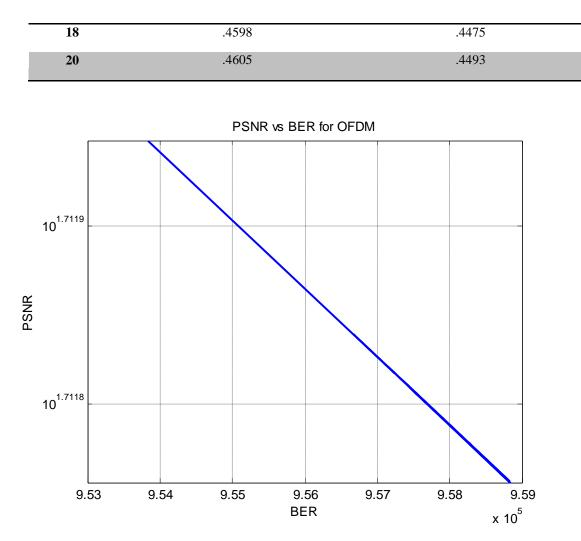
Figure 6-3-9 PSNR vs BER plot for transmitted and reconstructed image with OFDM
