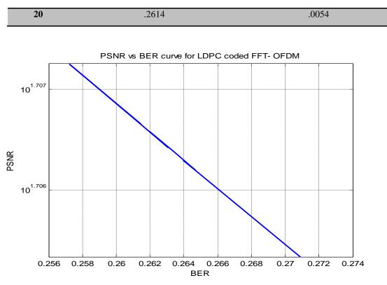
Figure 6-3-21 PSNR vs BER plot for transmitted and reconstructed image with LDPC coded FFT-OFDM
