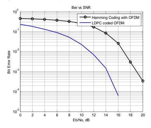
Figure 4-3-5 Performance Analysis of OFDM and LDPC coded OFDM with 128 FFT
