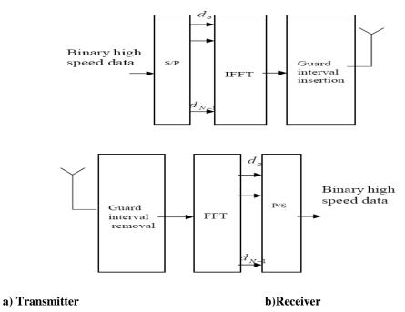
Figure 3-4-2 OFDM System Model
