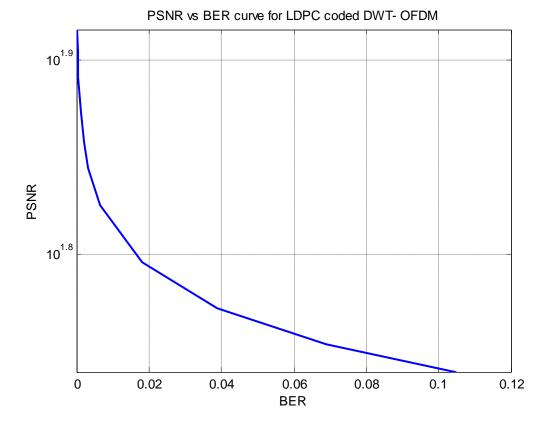
Figure 6-3-14 PSNR vs BER plot for transmitted and reconstructed image with LDPC coded DWT-OFDM
