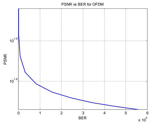
Figure 6-3-1 PSNR vs BER plot for transmitted and reconstructed image with OFDM
