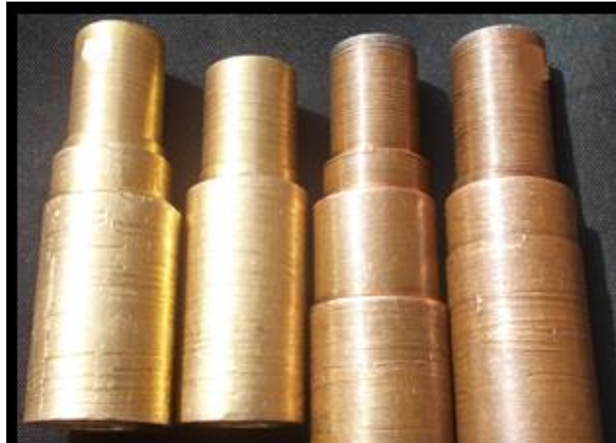
Figure 28 Brass and Copper tools (Cryogenic and Non-cryogenic)
