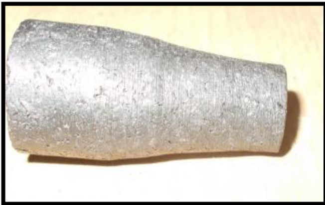
Figure 30 Non-Cryogenic Graphite tool
