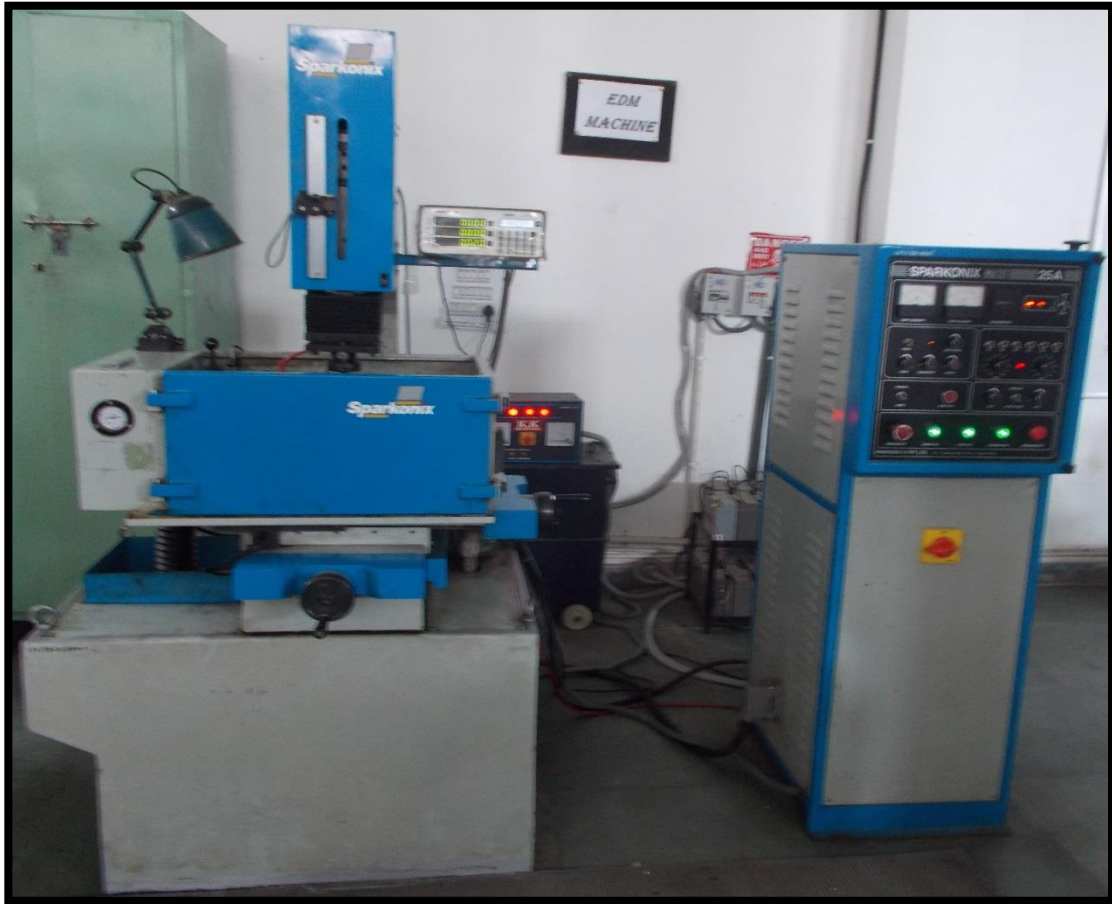
Figure 20 EDM set up
