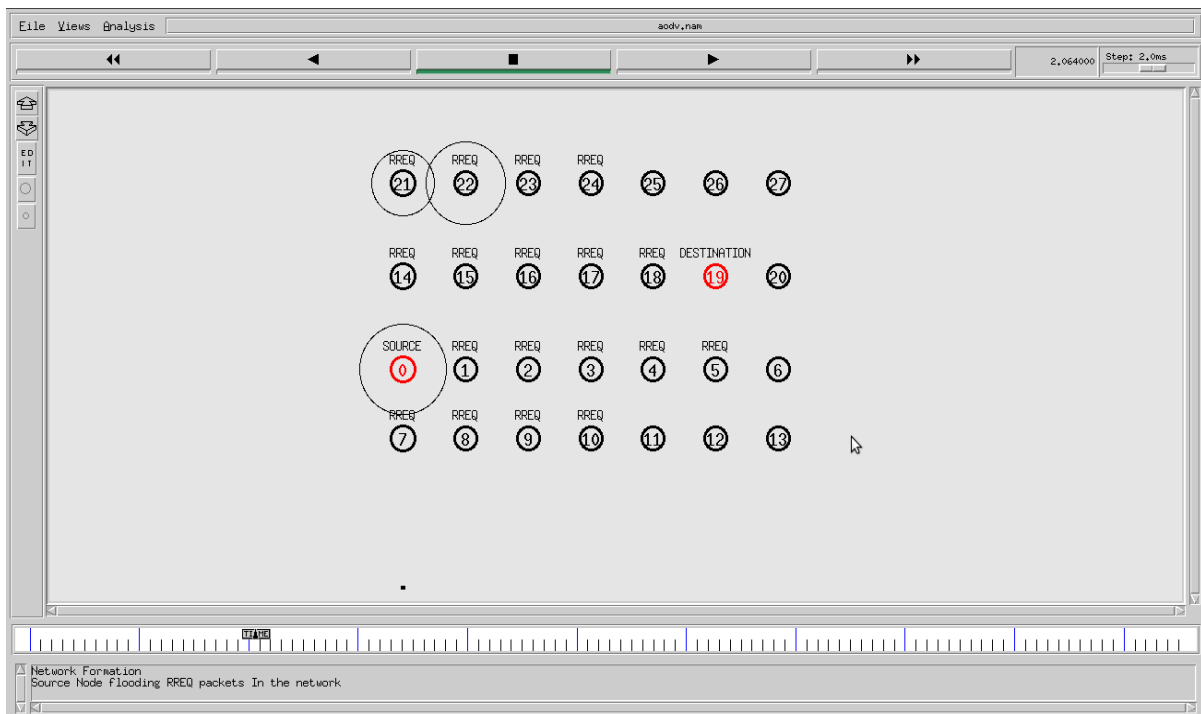
Figure 6.4 Route Request Flooding in the Network
