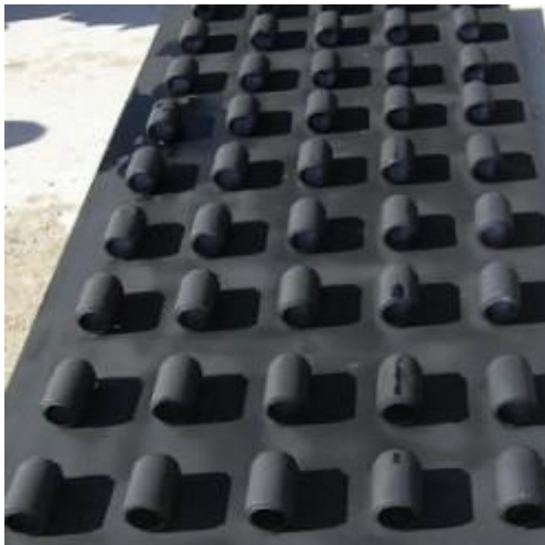
Figure 3.19 Absorber plate with Al cans arranged in transverse manner (Type II)
