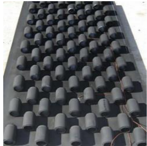
Figure 3.20 Absorber plate with Al cans arranged in transverse manner (Type I)
