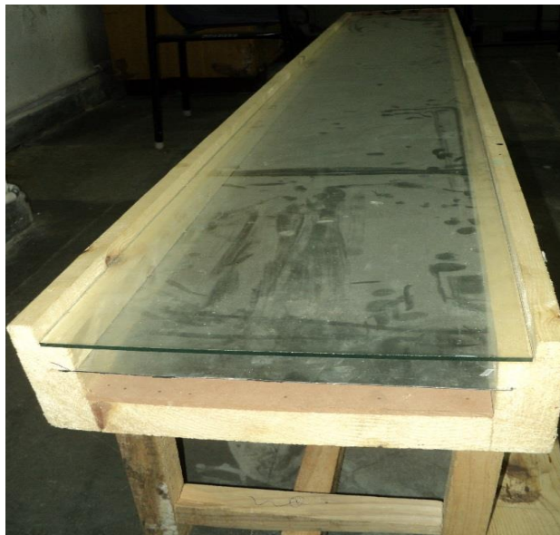
Figure 6.3 Pictorial view of rectangular duct
