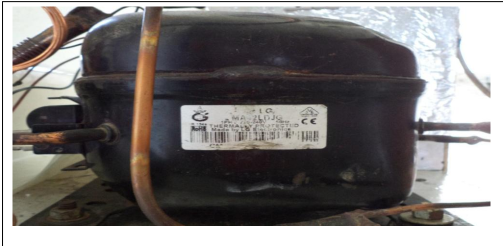
Figure 7.3: Hermetically sealed compressor
