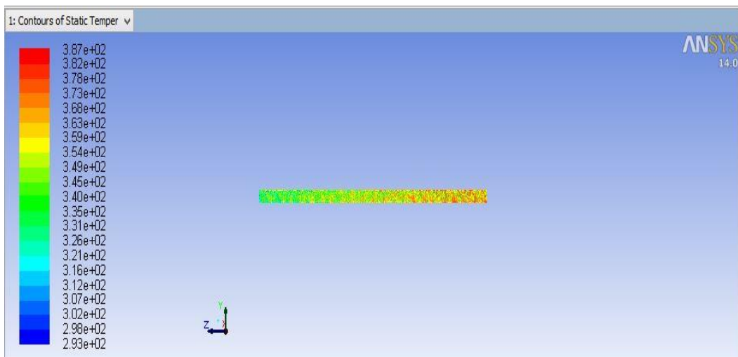
Fig. 7.12. Temperature of fluid inside the channel under pressure 35000 Pa and 900000 W/m 2 heat flux
