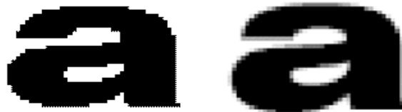
Figure 5.8 (a): Effect of Anti-aliasing
