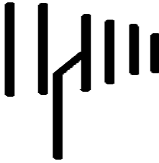
Figure 2.7 Yagi- Uda antenna array
