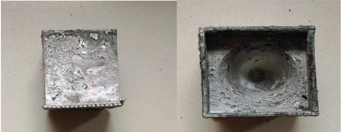
Figure 24 Burning of samples due to High Current
