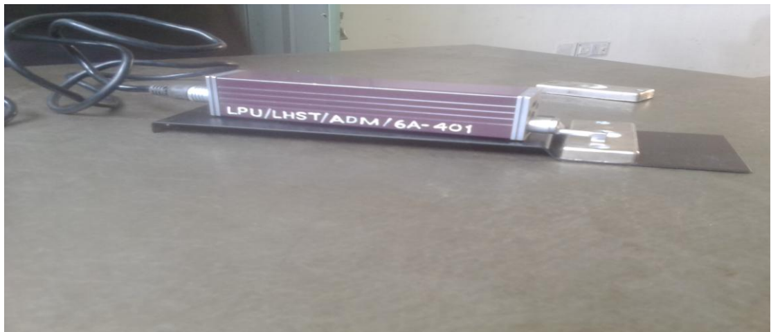
Figure 18 Measurement of Surface Roughness using Talysurf
