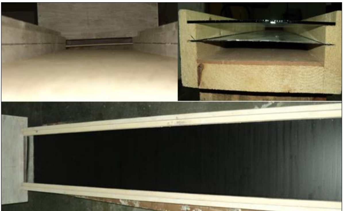
Figure 37 Pictorial view of solar air duct
