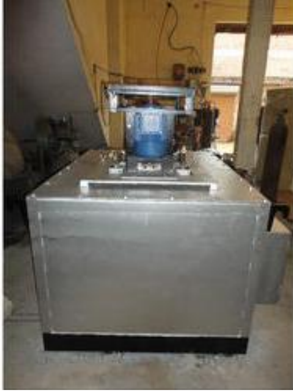
Fig15: Salt bath tempering furnace
