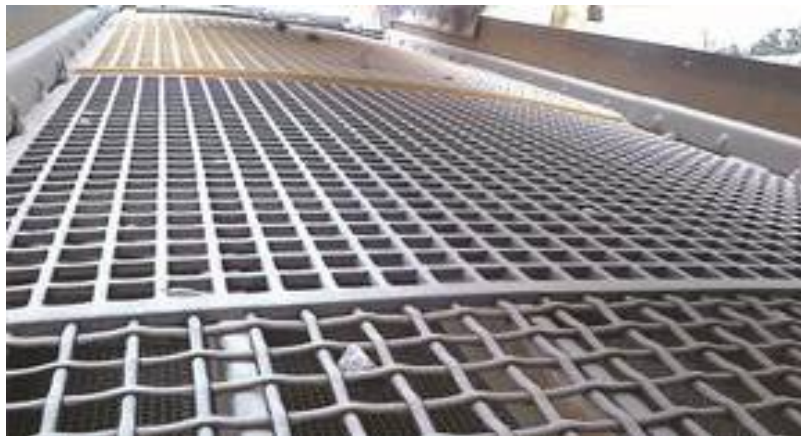
Fig. 3.3 Meshed bridge system
