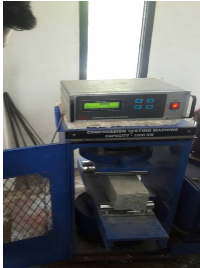
Figure: 17 Flexural strength test
