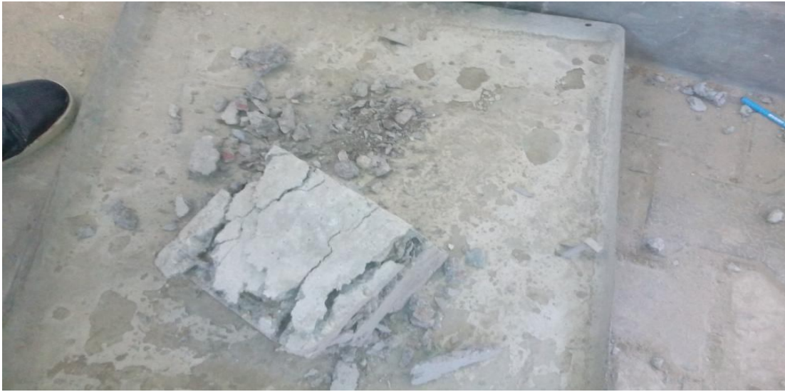
Figure 20: view of cube failed under the compressive load
