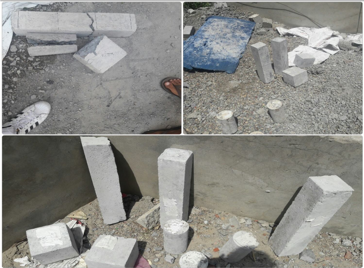
Figure 18: View of cubes before and after compressive load
