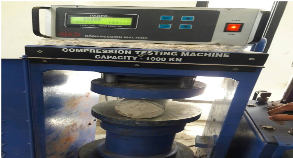
Figure 15: Split tensile strength test
