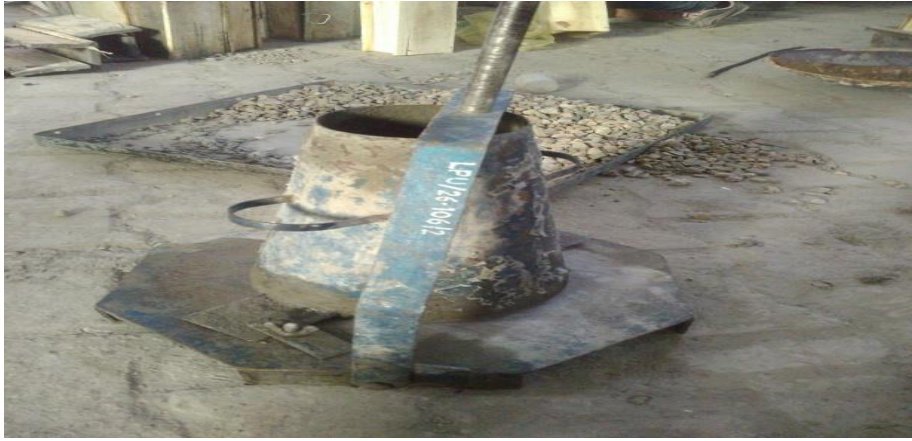
Figure: 9 Apparatus of Slump Cone Test
