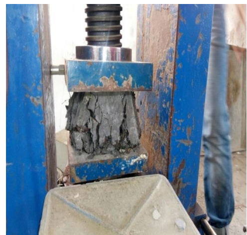
Figure:16 Failing of specimen
