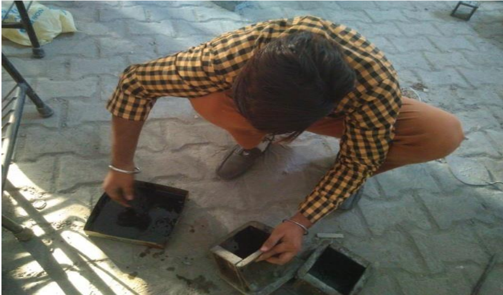
Figure: 4 Applying oil on inner surface of the moulds
