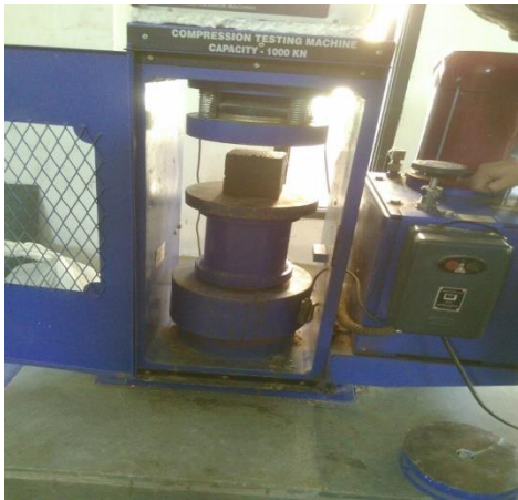
Figure:13 Placing of specimen on test plate
