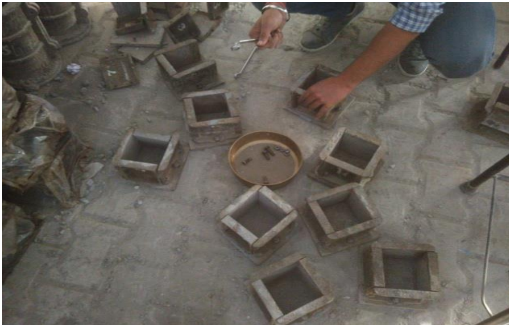
Figure: 3 Fixing cube with base plate
