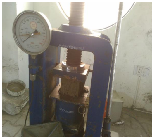
Figure:15 Specimen under compression
