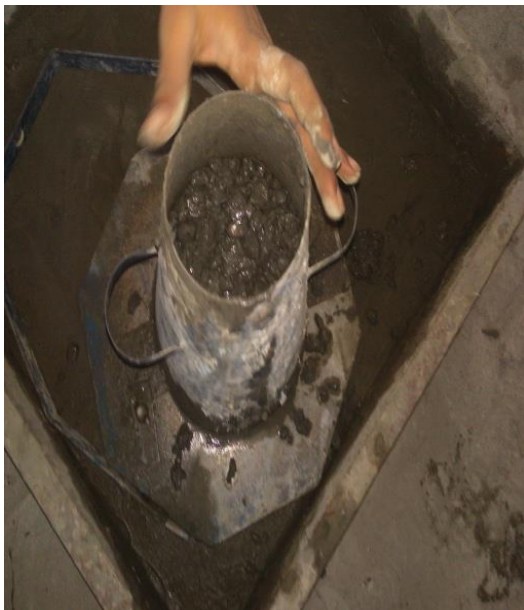
Figure:10 Layer by layer compaction
