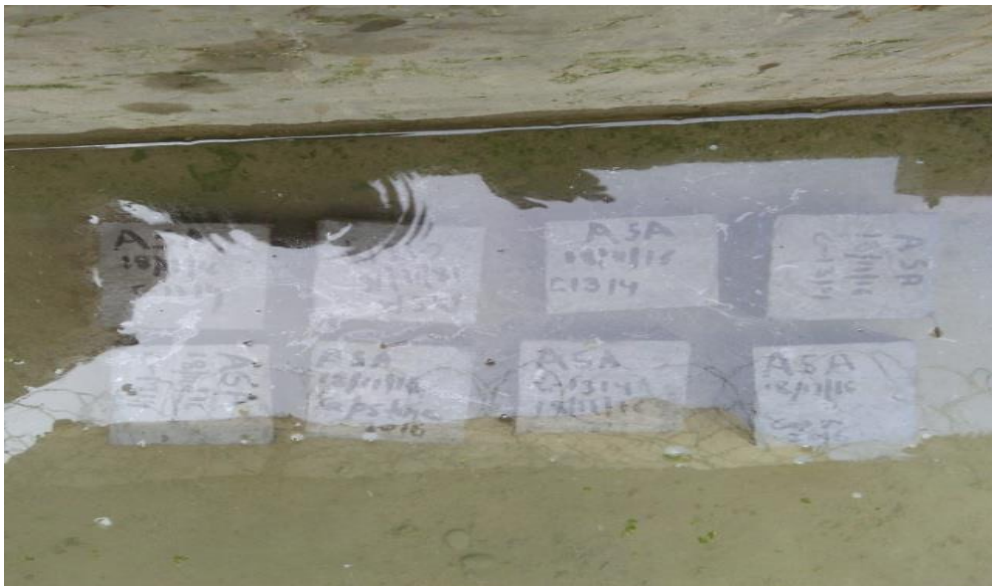
Figure: 8 Curing of cubes
