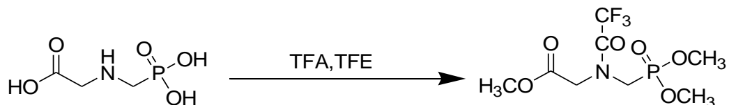
Figure 2.16 Derivatization of glyphosate with Mixture Of Trifluoroacetic Anhydride And Trifluoroethanol
