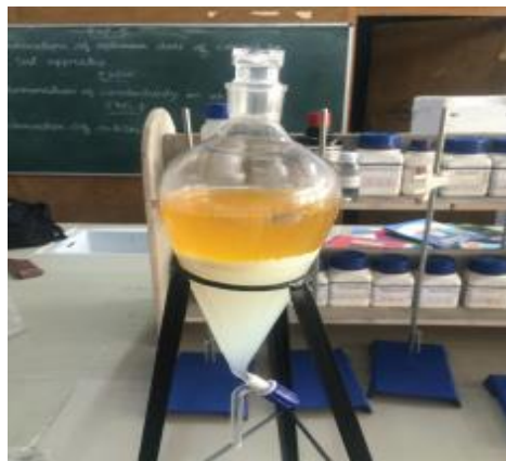
Figure 4.3 Formation of ester phase and glycerol
