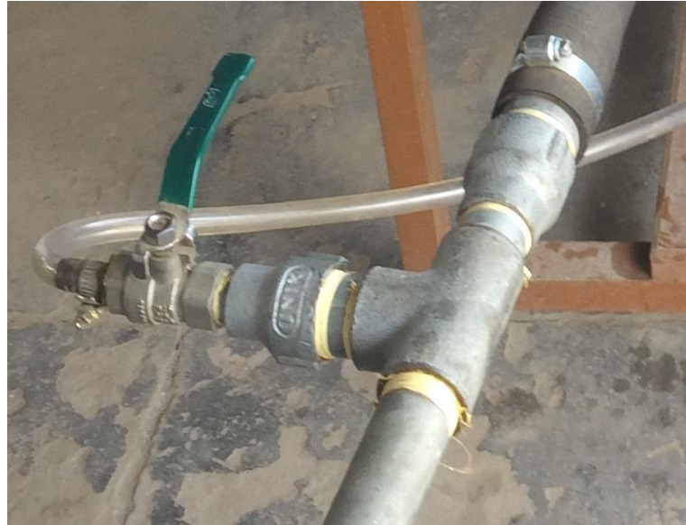
Figure 4.17 Modification of intake manifold of the engine
