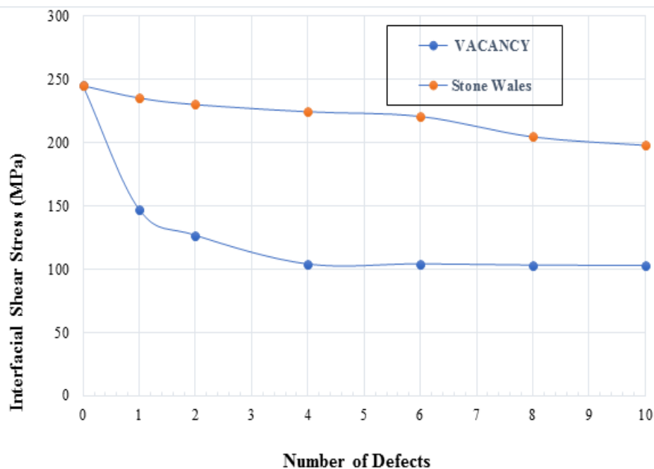
Figure 6.12 Comparison in interfacial shear stress between SW and Vacancy defect of SWCNT/NR composite with increase in number of defects
