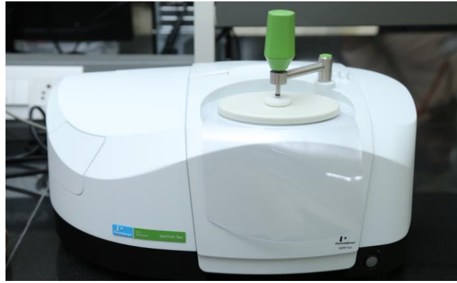
Figure 4.10 Fourier Transform Infrared Spectroscopy setup
