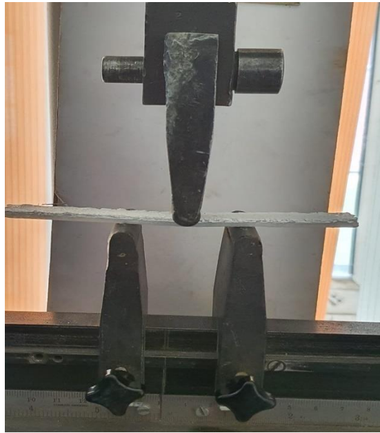
Figure 4.7 Schematic diagram of Flexural Testing
