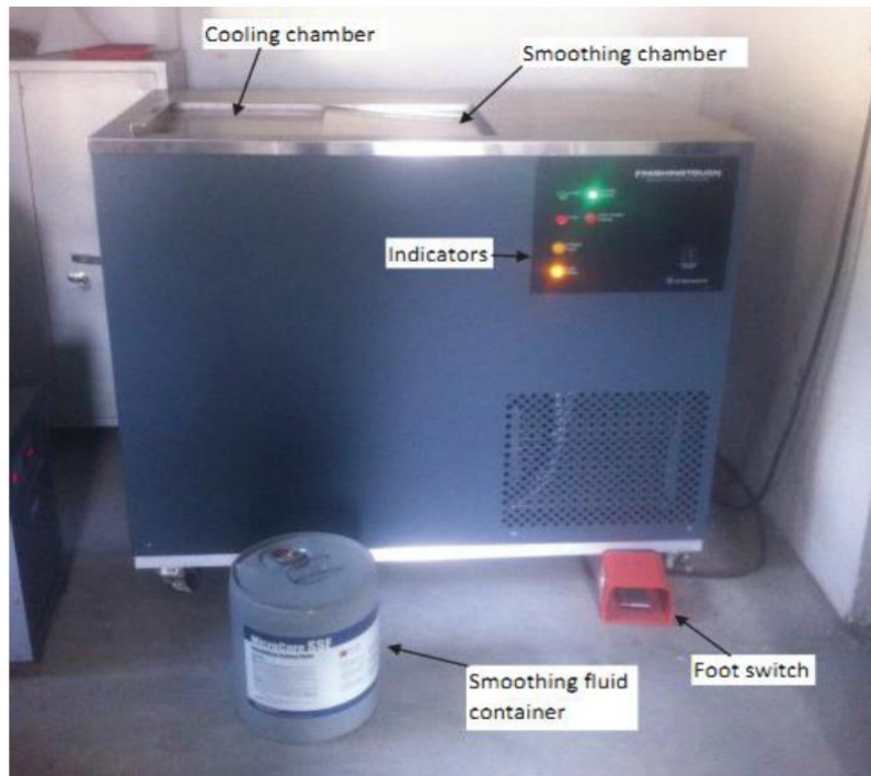
Figure 4.14 Chemical Vapor Smoothing station Setup
