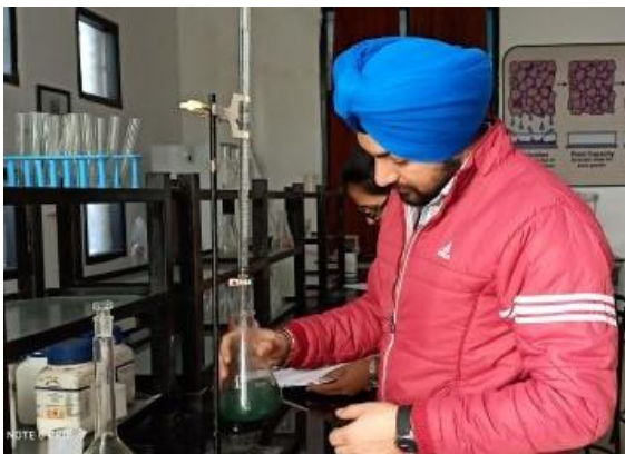
Plate 28: Organic carbon testing in soil samples indicating green colour
