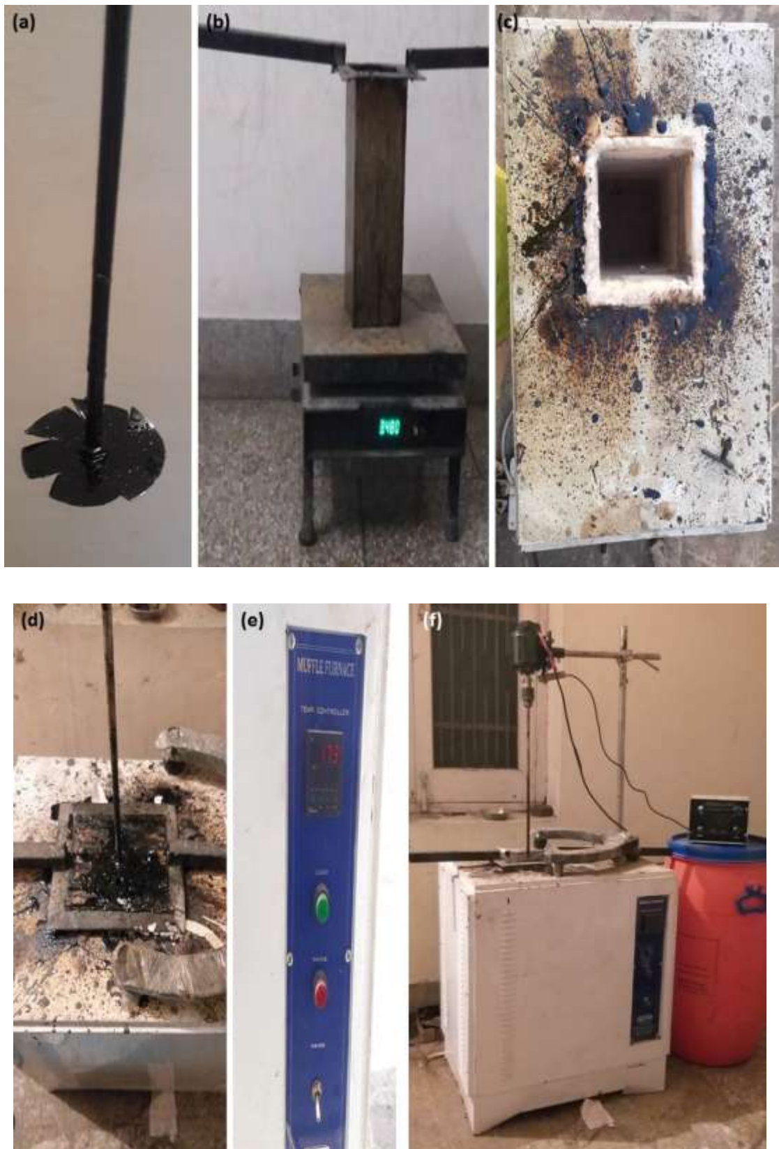
Figure 2.3: (a) Six blade mixer (b) Mixing vessel (c) Top view of furnace (d) Mixing vessel in the furnace (e) Front view of furnace (f) Fabricated apparatus
