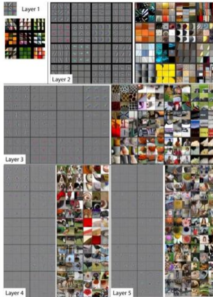
Fig. 3.14: Each layer of the neural network will extract specific features from the input image. (source: http://www.deeplearningbook.org )
