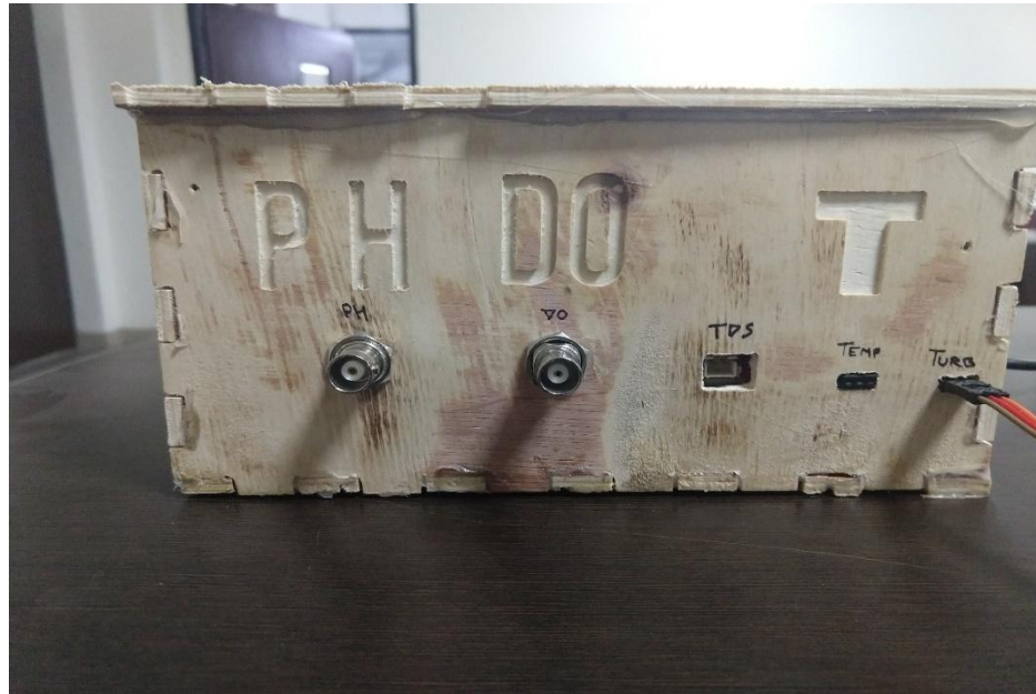
Figure 5.8 : Connectors for water quality sensors
