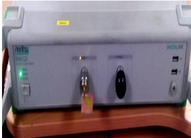
Fig. 3.12 Measurement of the antenna with MS46322A VNA
