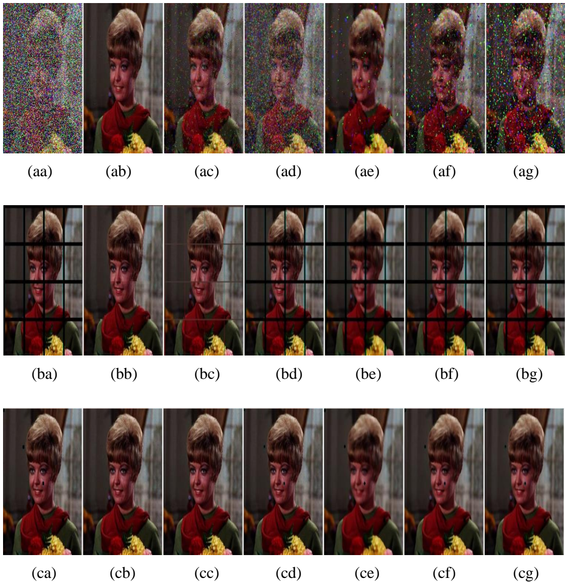
Figure 4.17. (a) Original color image, (aa) Color image corrupted by 50% Salt and Pepper noise, (ba) Color image corrupted by 6 pixel wide strip line artifact, (ca) Color image corrupted by 6*6 pixel size blotches artifacts,(ab–cb) Image restored using proposed method from (aa–ca), (ac–cc) Image restored using the ROAD-TGM from (aa–ca), (ad–cd) Image restored using the DBMF from (aa–ca), (ae–ce) Image restored using the CWMF from (aa–ca), (af–cf) Image restored using the PSMF from (aa–ca), (ag–cg) Image restored using the MF from (aa–ca). NB: ROAD-TGM, Rank-Ordered Absolute Differences Trimmed Global Mean Filter; CWMF, Center Weighted Median Filter; DBMF, Decision-Based Median Filter; PSMF, Progressive Switching Median Filter; and MF, Median filter.
