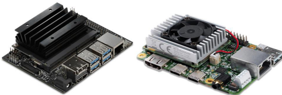
Figure 4.3. Embedded boards a). NVIDIA’s Jetson Nano b). Google Coral’s Dev Board
