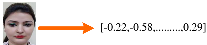
Figure 4.8. Generation of the 128-d real-valued number feature vector of each training image in the dataset
