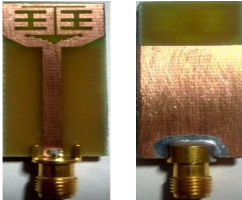
Figure 4.17: The fabricated structure of Ant 4 (a) Front end (b) Back End
