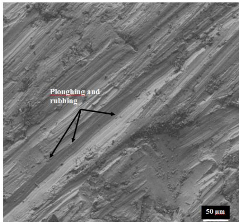
Fig. 5.26. SEM images of worn-out surface of pin against WC counter surface
