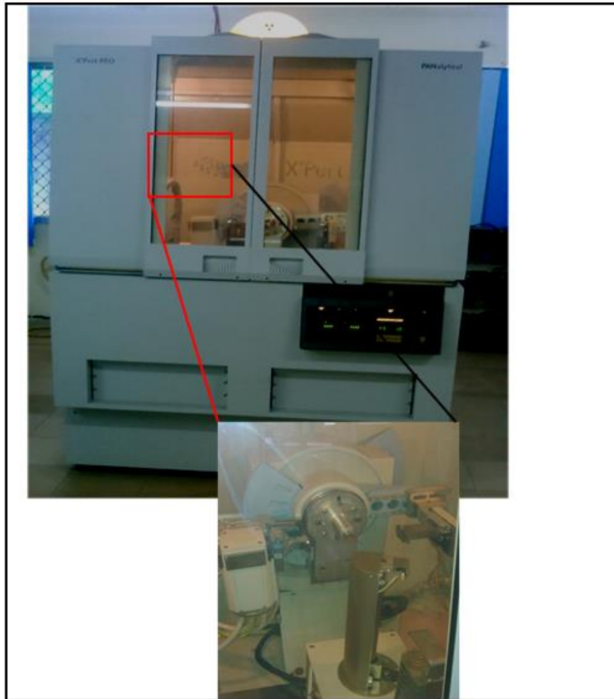
Fig. 4.14. XRD equipment for Phase Composition Analysis
