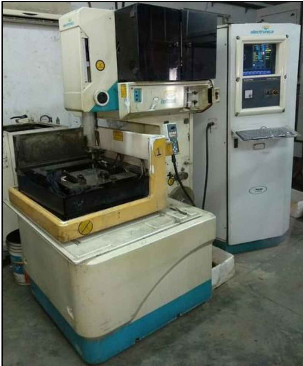
Fig. 4.8. Photograph of Wire-electric discharge machining (W-EDM) process
