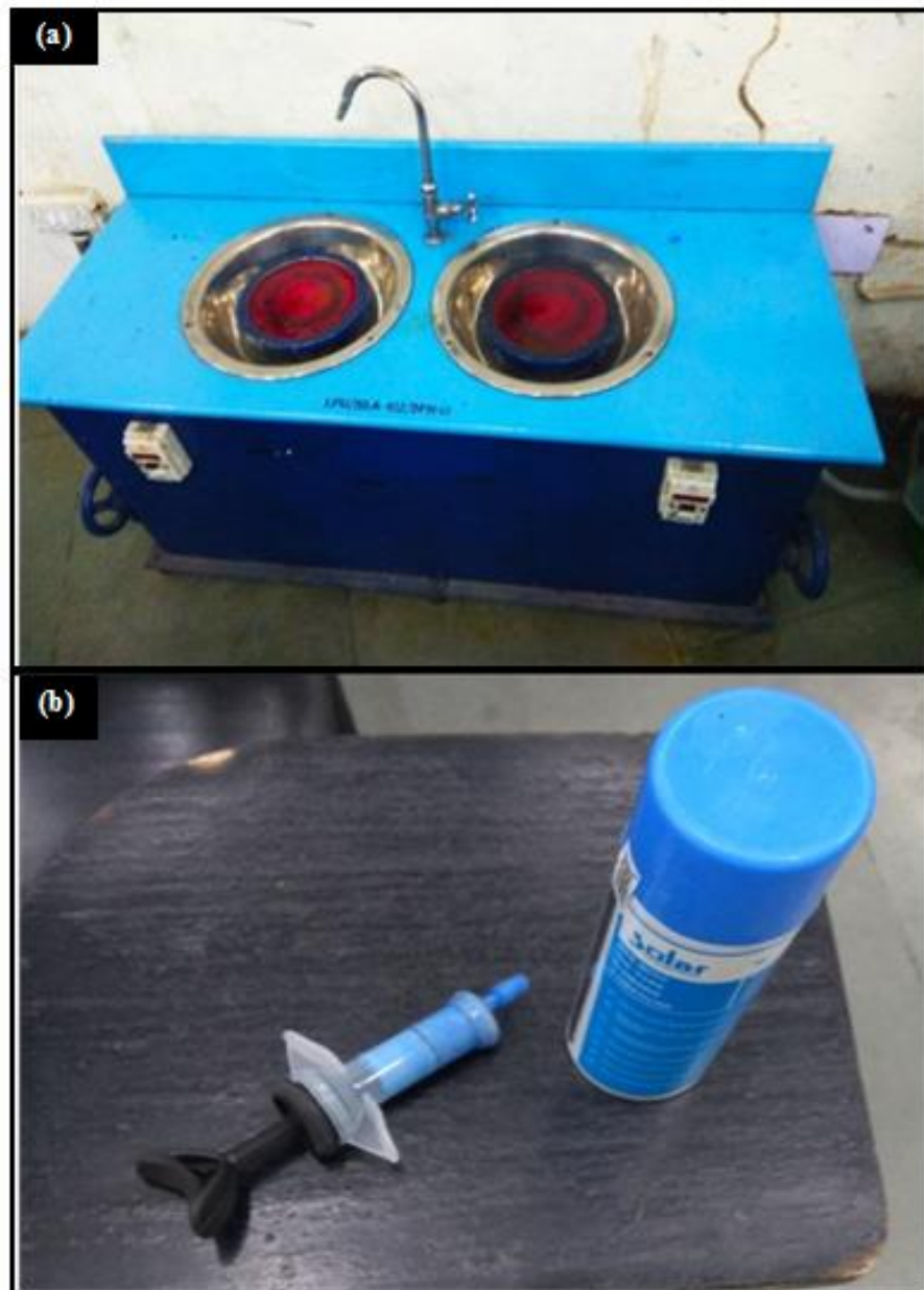
Fig. 4.9. (a) Disc polishing machine; (b) Diamond syringe & Developer
