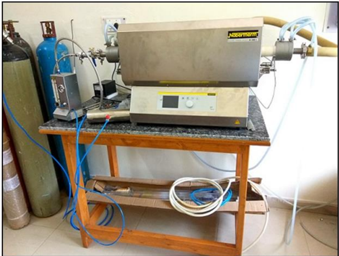
Fig. 4.10. Experimental set-up of thermo-chemical diffusion
