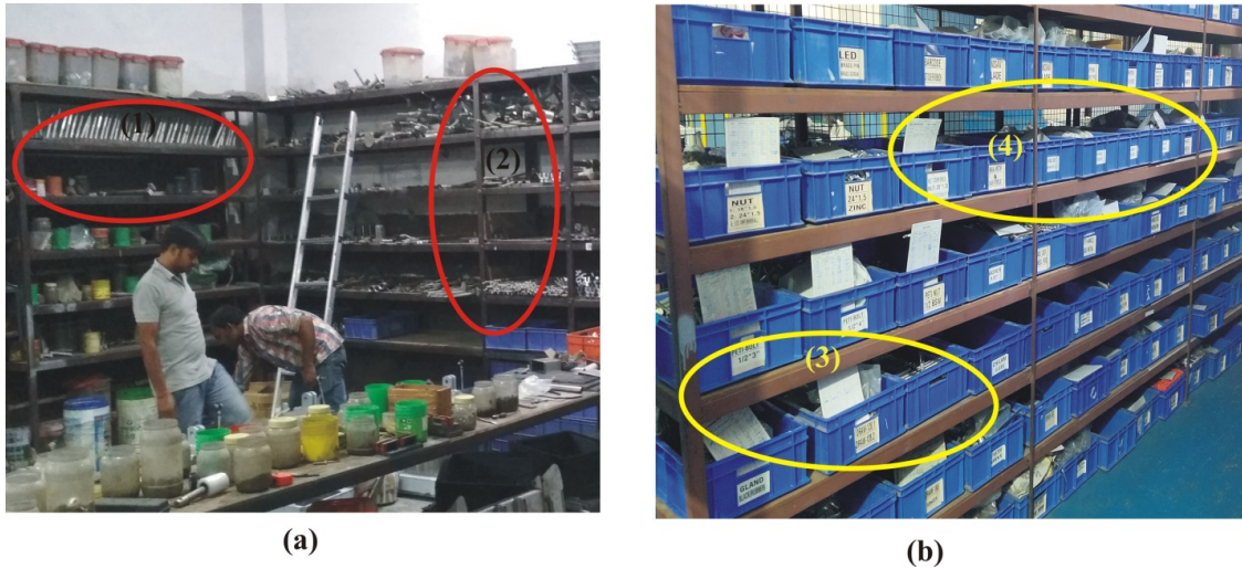
FIGURE 6.12: (a) Assembly section before 6S adoption; (b) Assembly section after 6S adoption.
