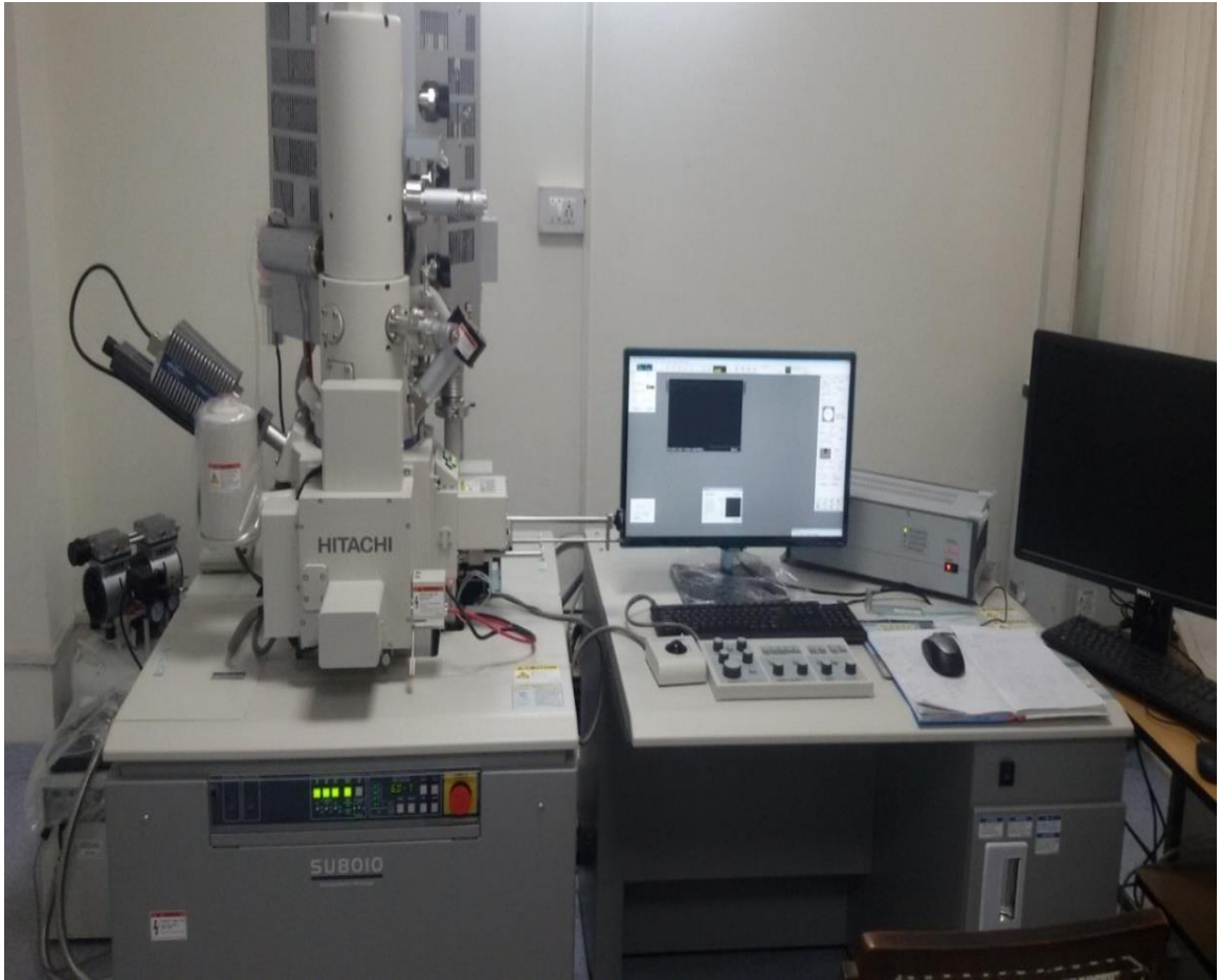
Figure 4.8. Field Emission Scanning Electron Microscope (FE-SEM) with EDS (Brand: HITACHI, Model: SU8010)
