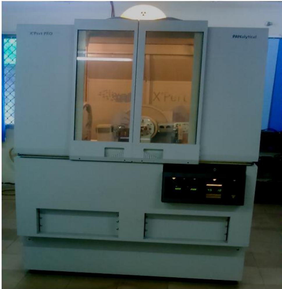
Figure 4.9. XRD equipment for Phase Composition Analysis, Brand: X'pert-PRO, PANalytical, Almelo, The Netherlands
