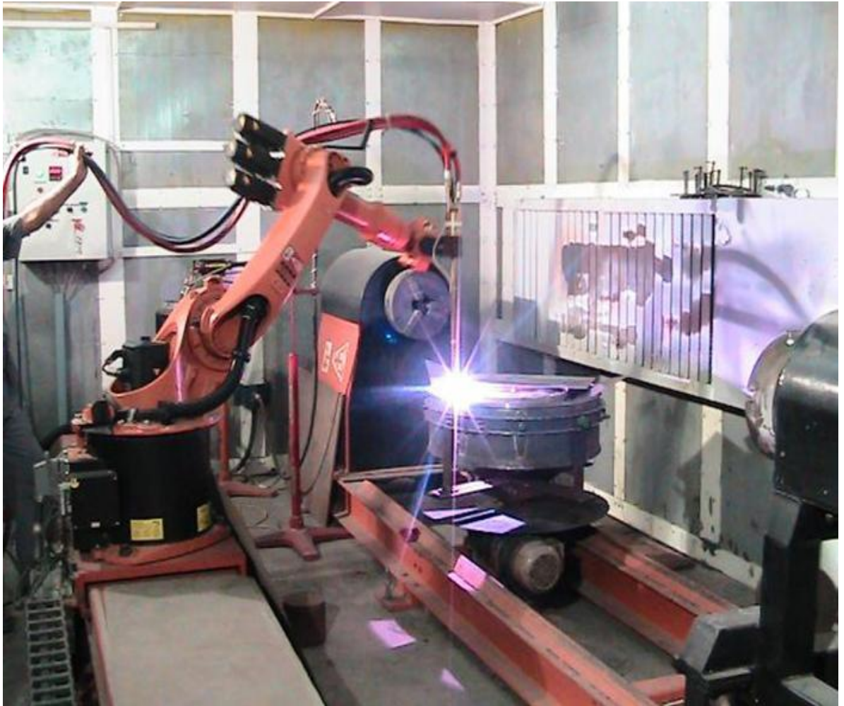
Figure 4.6. Experimental set-up of plasma Spray Deposition process
