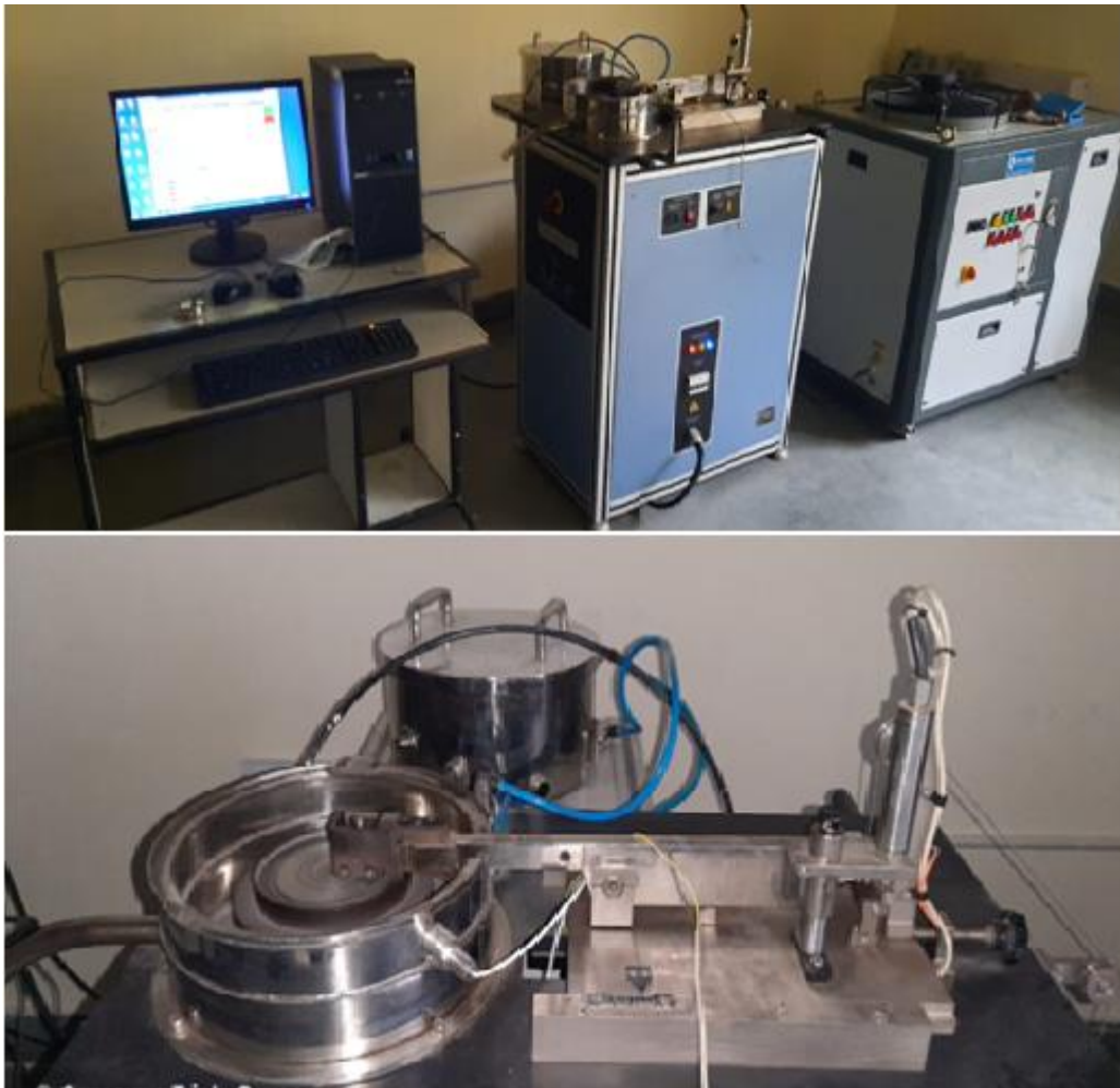
Fig. 3.5 High-temperature pin-on disc tribometer used for testing coated specimens at various conditions.
