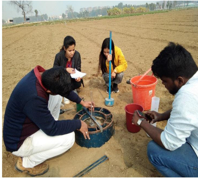
Plate 1 Estimation of infiltration rate and bulk density
