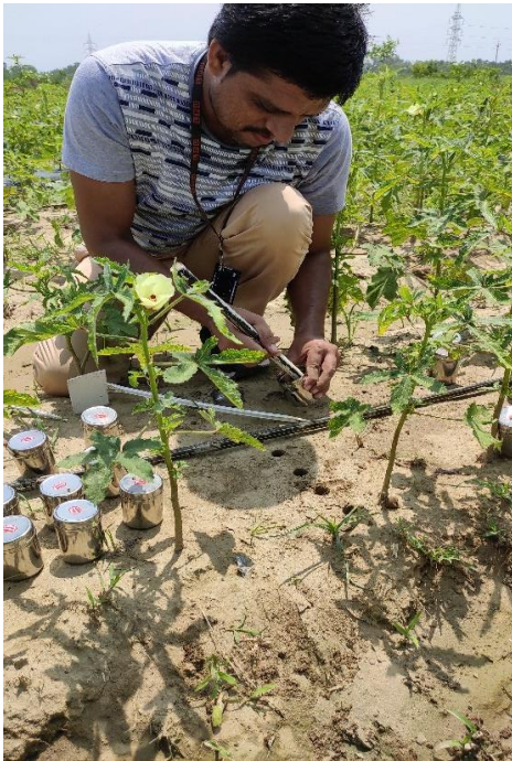
Plate 5 Soil sampling for soil moisture determination
