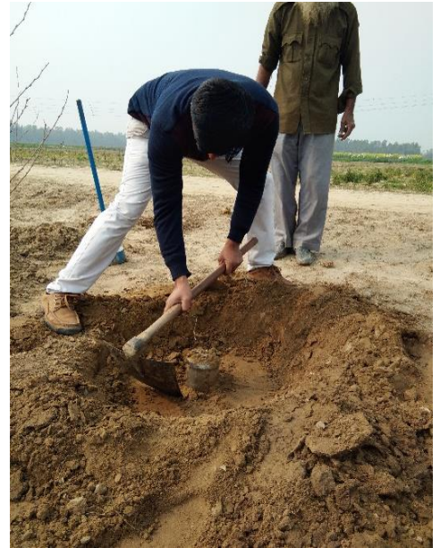
Plate 1 Estimation of infiltration rate and bulk density
