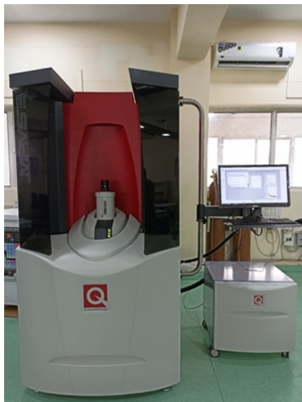
FIGURE 4.7: Quantum Design MPMS3 (SQUID) Superconducting Quantum Interference Device Magnetometer at IIT Roorkee
