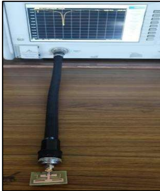
Figure 3.22: Fabricated antenna with vector network Analyzer for |S_{11}| (dB) measurement.
