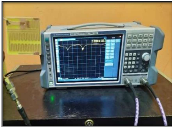
Figure II.3: The photograph of the VNA which is used to measure the return
