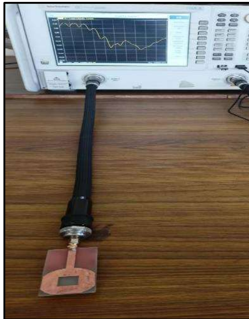
Figure 3.10: Fabricated antenna with vector network Analyzer for |S_{11}| (dB) measurement.
